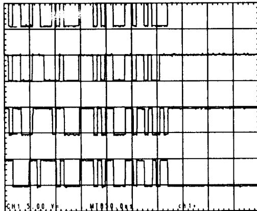
IC101 pin 30 (DATA) for TV tuner channels 2, 4, 6 and 7 (from top to bottom). 5V/DIV. TB 50μSEC/DIV.
