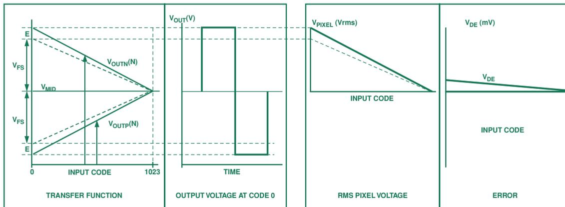
Figure 3. A typical case of  $V_{DE}$  or differential error. From left to right, plots show transfer function, time-domain rms signal at code zero, rms voltage as seen by the pixel, and the error vs. DAC code.
