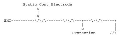
If the EHT rises too high, then the voltage at the protection point also rises, and a shutdown signal is sent to the scan processor.
