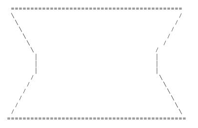
In particular, this sounds like a pincushion problem - to correct for pincushion, a signal from the vertical deflection that looks something like a rectified sinewave is used to modify width based on vertical position. There is usually a control to adjust the magnitude of this signal and also often, its phase. It would seem that this circuit has ceased to function.
