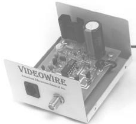
Receive board mounted in enclosure
