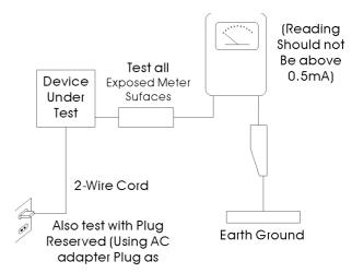
**AC Leakage Test**
