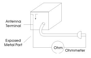
Insulation Resistance Test
