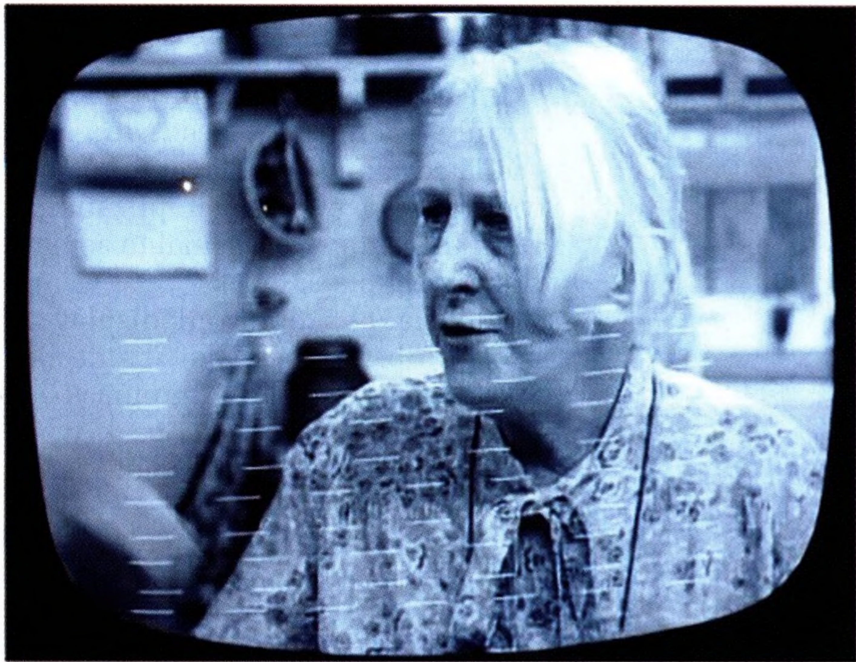
The diagonal white lines often seen on older sets are retrace lines, which are normally hidden but can manifest themselves due to the VBI not being fully blanked. By the way, the blue cast on these screens is quite typical for sets of the day.
