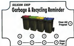
Fig.3 (above): this front-panel artwork can be used as a drilling template for the case lid. It can either be copied or downloaded from the SILICON CHIP website and printed out. The photograph at right shows the M3 x 15mm standoffs and the two extra M3 nuts at each corner mounting position.
