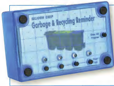
The front panel label sits inside the lid of the translucent blue case. The unit is easy to program and has very low current drain, with a battery life of up to three years.
