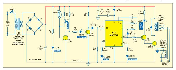
rectly from the bridge rectifiers. When 'on'/'off' switch S1 is closed, LED1 glows to indicate that the circuit is powered 'on.'
