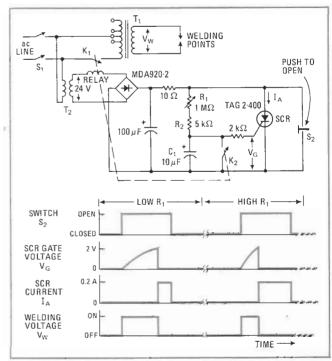
**Welding made easy.** When  $S_2$  is pushed open, welding current flows and gate voltage starts to rise. Once gate voltage becomes high enough to let SCR conduct, welding current ceases. SCR continues to conduct until operator allows  $S_2$  to close; thus, duration of welding pulse is determined only by charging time for  $V_G$  to reach SCR firing voltage, not by how long  $S_2$  is open.
