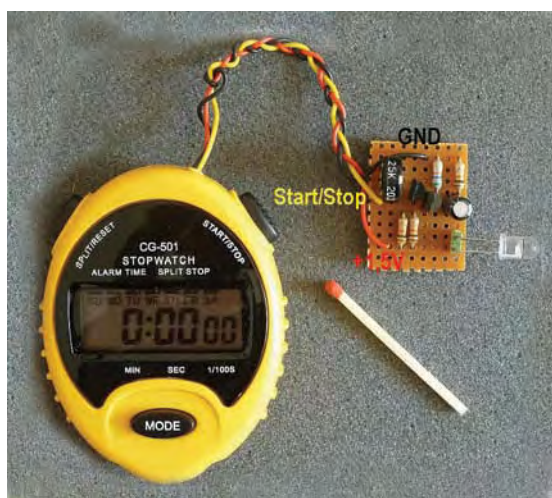
Figure 1 You build the circuit on a small prototype board that connects to the CG-501 stopwatch.
