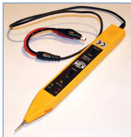
Fig.8.4. A typical logic probe
