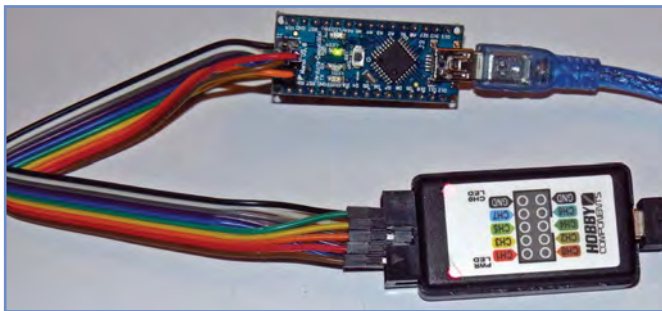
Fig.8.21. Connecting the low-cost logic analyser to a Node MCU microcontroller
