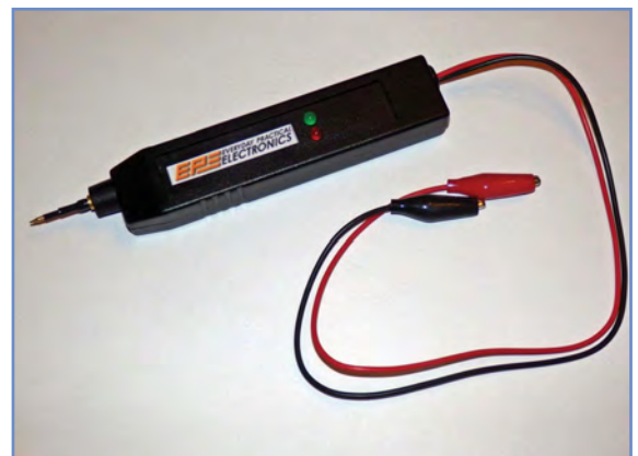
Fig.8.30. External appearance of the simple logic probe
