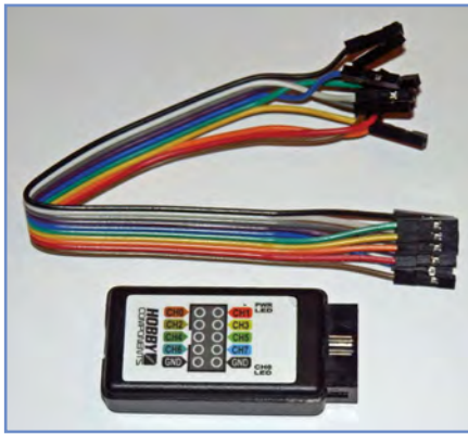
Fig.8.20. Ultra-low-cost 8-channel USB logic analyser
