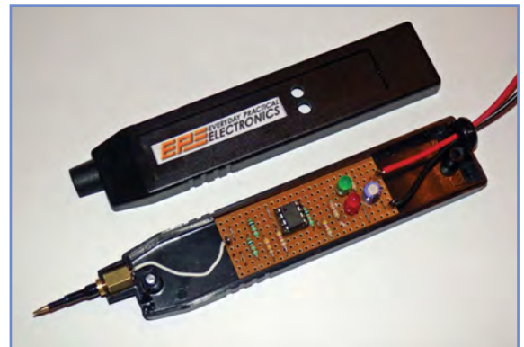
Fig.8.29. Internal wiring of the simple logic probe
