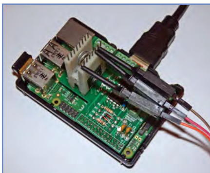
Fig.8.25. Using an IC test clip to check logic signals present on a Raspberry Pi expansion board
