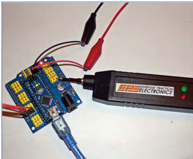
Fig.8.32. Typical supply lead connections. On this Nano breakout board the red crocodile clip is taken to '3V3' and the black is taken to 'GND'
