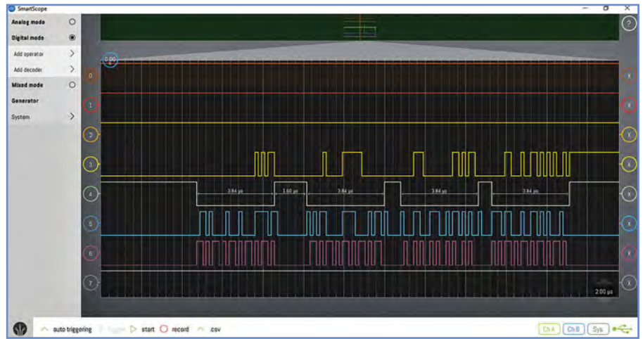
Fig.8.18. Captured digital data using LabNation's SmartScope software
