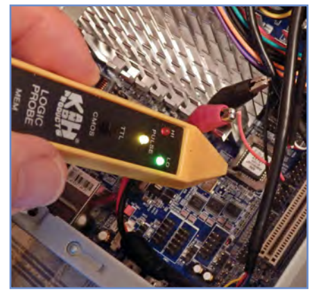
Fig.8.8. Using a logic probe to check the signals present on the BIOS chip of a Mini-ITX motherboard. The probe indicates a signal that is mostly low but also pulsing high (see Fig.8.6)
