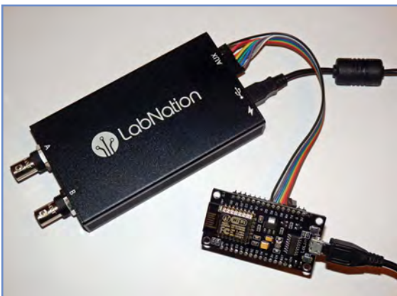
Fig.8.17. A USB digital storage 'scope with auxiliary digital inputs connected to digital I/O lines on a Node MCU microcontroller
