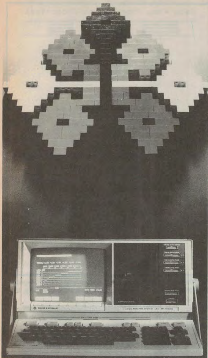
The LAS logic analyser system from Rohde & Schwarz, capable of both state and timing analysis as required.
