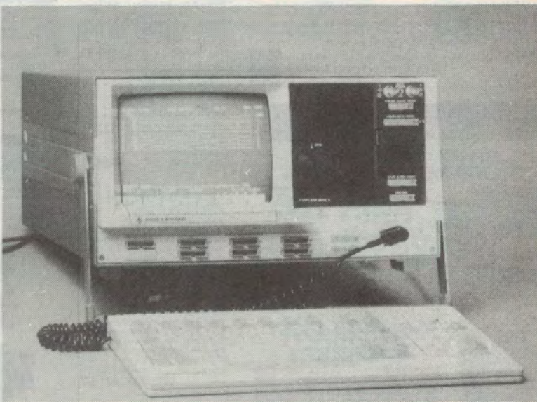
Conventional test instruments like a voltmeter or oscilloscope (left) are of limited use in checking logic circuits. A logic analyser like that at right is much more suitable.
