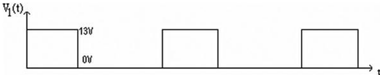
Figure 4.18 Output of the rectifier.
