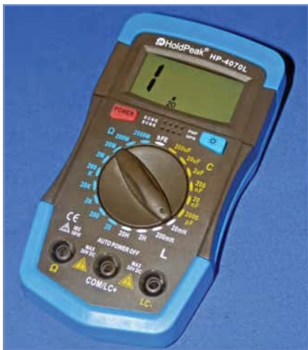
Fig.5.4 A low-cost multi-range LCR meter
