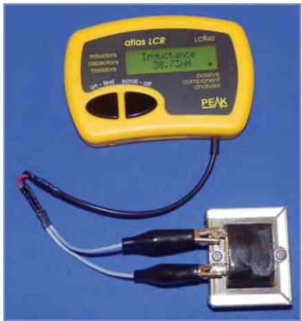
Fig.5.5 The Peak Electronics LCR40 being used to check the value of a small steel-cored inductor
