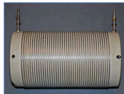
Fig.5.11 A large air-cored 44 \mu H inductor wound on a low-loss ceramic former
