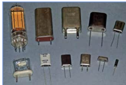
Fig.5.14 A selection of crystals with fundamental resonant frequencies of 32kHz to 18MHz
