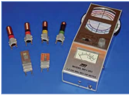
Fig.5.12 A wide-range dip meter covering 1.5MHz to 250MHz in six ranges
