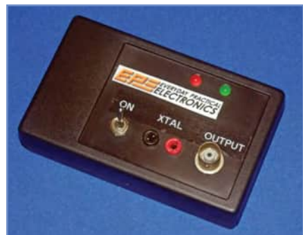
Fig.5.19 External appearance of the finished Handy Crystal Checker
