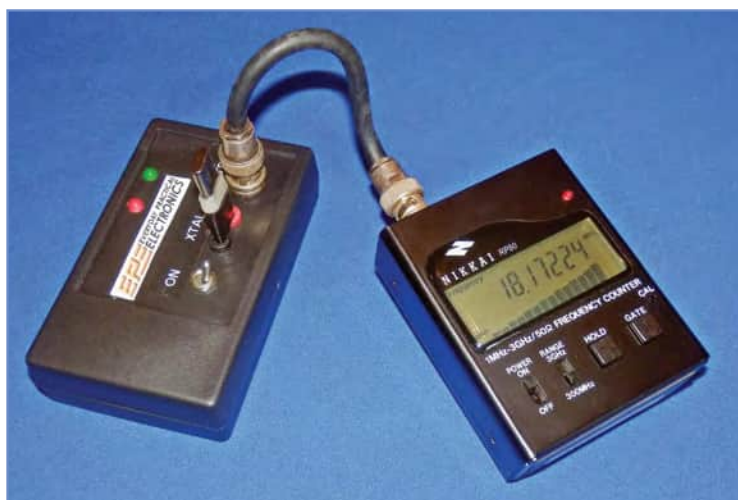
Fig.5.22 Using the breadboard test fixture to test a wire-ended HC6 crystal
