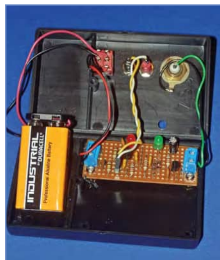
Fig.5.18 Internal wiring of the Handy Crystal Checker
