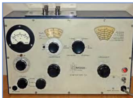
Fig.5.9 An Advance Electronics T2 Q-meter
