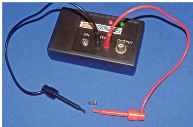
Fig.5.20 Using the Handy Crystal Checker to check a wire-ended crystal
