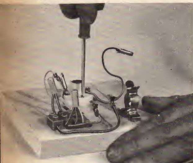
Mounting the m.e.s. bulb holder on the baseboard
