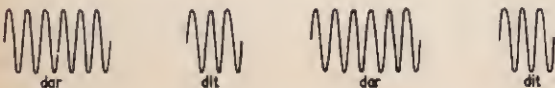
Fig. 22.2a. A continuous wave of oscillations is broken up into long and short bursts by a morse key
