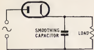
Fig. 4. A.C. rectification (left)
