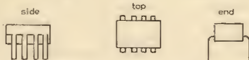
1.1 Outline shape of a typical 8-pin dual-in-line integrated circuit, about \frac{1}{2} times actual size.
