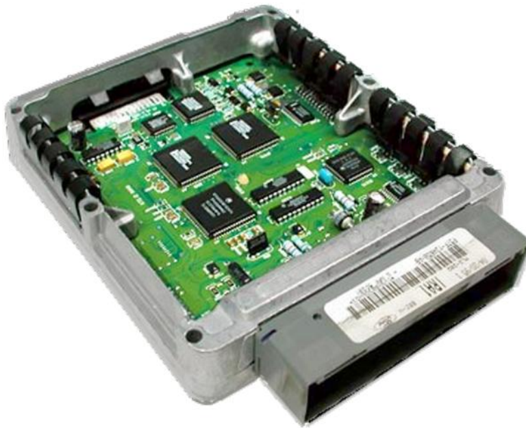
A typical example of a control unit, usually located in the engine area or in the cabin.
