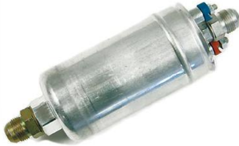
Centrifugal electric fuel pump
