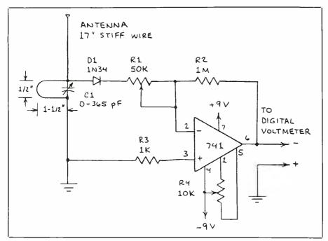
Fig. 5. A radio-frequency field-strength meter.
