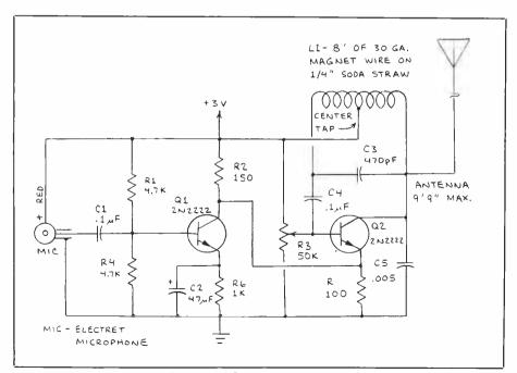
Fig. 2. A low-power broadcast-band voice transmitter.
