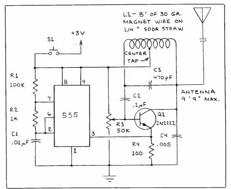
Fig. 1. A low-power broadcast-band tone transmitter.
