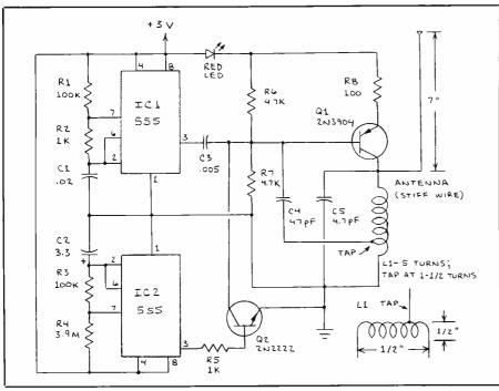
Fig. 3. A low-power vhf pulse transmitter.
