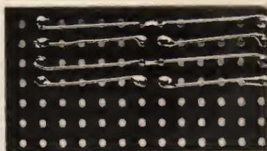
Fig. 4a. Plain perforated s.r.b.p. sheet with copper wire connections and soldering pins
