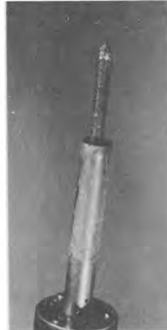
Figure 1a It is important to keep your soldering iron clean at all times. This illustration shows a dirty, corroded bit that would certainly not aid you in obtaining a clean, secure joint.
