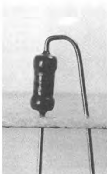
Figure 5: The correct method of upright installation when the hole spacing is restricted. Note in particular how the lead has been bent.
