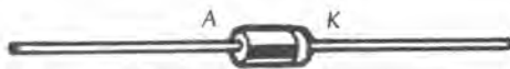
A typical diode with a band at one end to indicate the cathode (K).
