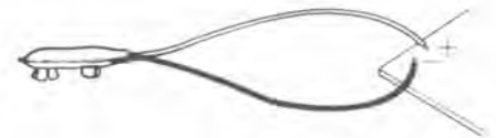
Figure 5a: Basic 'battery snap' wiring without switch. The black lead in all cases is negative.
