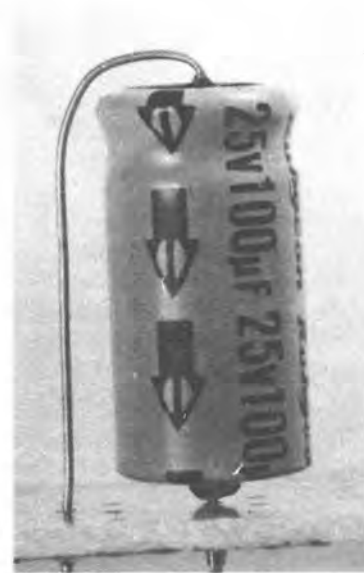
Figure 6: This is an example of an axial lead capacitor mounted in the upright position. When mounting electrolytic capacitors special care must be taken to ensure correct polarity.
