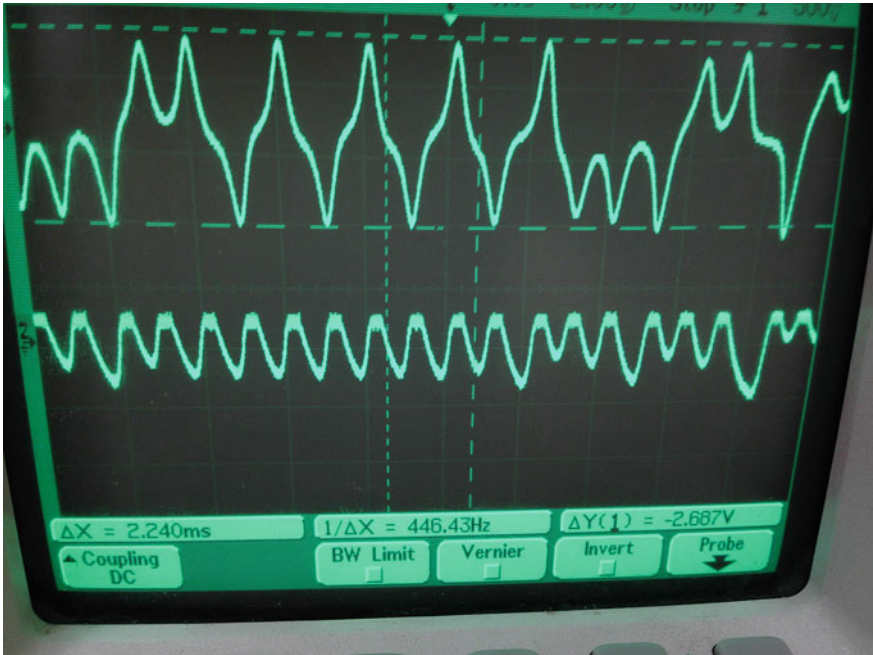
Fig. 3.4 x(t) from the Lorenz attractor realization on the FPGA, compared to z(t) . Notice the large variations in z(t) values are not being adequately captured by our digital system
