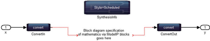
Fig. C.10 We need a SynthesisInfo block for controlling synthesis flow. By using the default option of Scheduled, we let DSP builder use a pipelining and delay distribution algorithm that create fast hardware implementations from an easily described untimed block diagram
