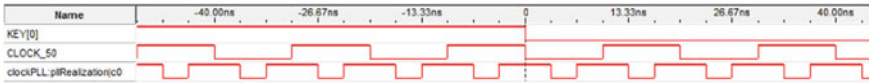
Fig. 3.16 Results from the SignalTap session. Notice how the 100MHz clock has twice the frequency of the 50MHz clock. Since we are not using a global reset, the signals are not synchronized
