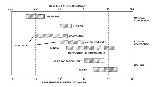
**Figure 11.4** Heat transfer coefficient for various heat removal/cooling techniques. (*From* [3]. *Used with permission*.)
