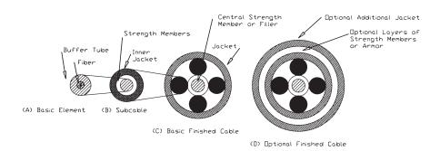
**Figure 19.4** In the breakout type of cable, each element is surrounded by a flexible strength member, which is then surrounded by an inner jacket. This forms a subcable, which is incorporated into a larger cable. Optional additional jackets or armor can be applied.
