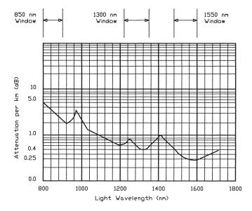
**Figure 19.2** Fiber attenuation vs. light wavelength characteristics. Attenuation has been reduced steadily in the last two decades through improved fiber drawing techniques and a reduction in impurities. It has now approached the theoretical limits of silica-based glass at the 1,300 and 1,550 nm wavelengths.
