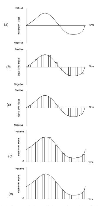
**Figure 17.1** Pulse amplitude modulation waveforms: (a) modulating signal; (b) square-topped sampling, bipolar pulse train; (c) topped sampling, bipolar pulse train; (d) square-topped sampling, unipolar pulse train; (e) top sampling, unipolar pulse train.
