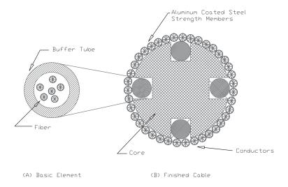
**Figure 19.6** Utility companies sometimes use an optical power ground wire type of cable because it incorporates a metallic power ground wire within the design. The cable is based on a slotted-core configuration, but with the addition of helically wrapped wires around the outside for strength and conductivity.
