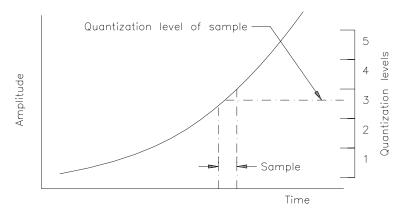
Figure 17.4 The quantization process.
