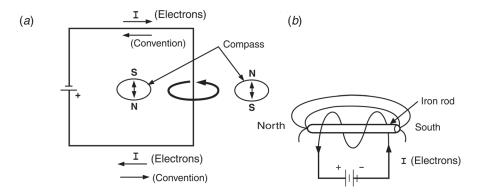
**Figure 9.2** Magnetic field surrounding a current-carrying conductor: (a) Compass at right indicates the polarity and direction of a magnetic field circling a conductor carrying direct current. *I* indicates the direction of electron flow. Note: The convention for flow of electricity is from + to –, the reverse of the actual flow. (b) Direction of magnetic field for a coil or solenoid.
