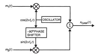
Figure 15.6 Simplified QAM modulator. (From [1]. Used with permission.)
