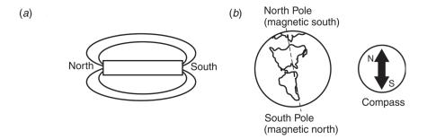
**Figure 9.1** The properties of magnetism: (a) lines of force surrounding a bar magnet, (b) relation of compass poles to the earth's magnetic field.
