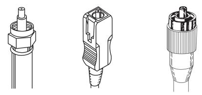
Figure 19.9 Common types of fiber-optic connectors.
