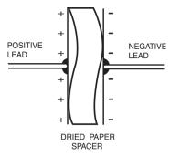
**Figure 8.6** Failure mechanism of an electrolytic capacitor exhibiting a loss of capacitance. After the electrolyte dries, the plates can no longer come in contact with the aluminum oxide. The result is a decrease in capacitor value.
