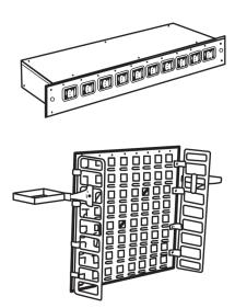
Figure 18.4 Data network patch-panel hardware.
