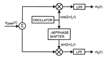
Figure 15.7 Simplified QAM demodulator. (From [1]. Used with permission.)
