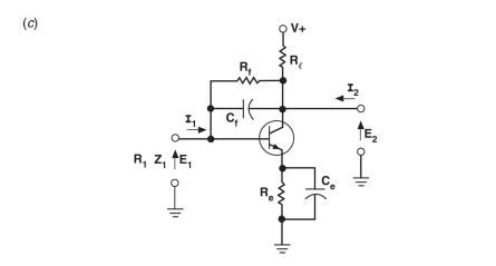
**Figure 13.1** Single-stage amplifier circuits: (a) common-emitter NPN, (b) common-source n-channel FET, (c) single-stage with current and voltage feedback.
