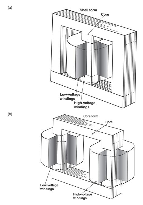
**Figure 9.4** Physical construction of a power transformer: (a) E-shaped device with the low- and high-voltage windings stacked as shown, (b) construction using a box core with physical separation between the low- and high-voltage windings.
