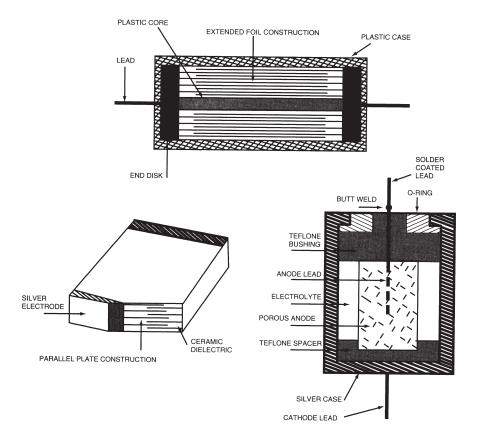
Figure 8.1 Construction of discrete capacitors. (From [1]. Used with permission.)
