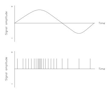
Figure 17.3 Pulse frequency modulation.
