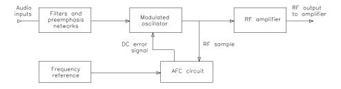
Figure 16.5 Block diagram of an FM exciter.
