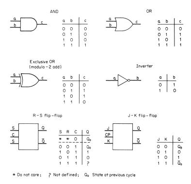
Figure 14.7 Basic logic circuits and truth tables.
