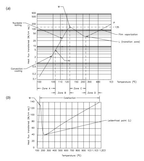
Figure 11.2 Nukiyama heat-transfer curves: (a) logarithmic, (b) linear.
