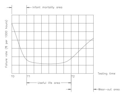
**Figure 20.2** The statistical distribution of equipment or component failures vs. time for electronic systems and devices.
