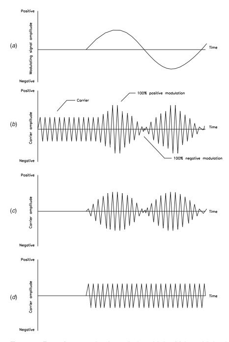
**Figure 15.5** Types of suppressed carrier amplitude modulation: (a) the modulating signal, (b) double-sideband AM signal, (c) double-sideband suppressed carrier AM, (d) single-sideband suppressed carrier AM.
