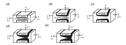
**Figure 12.5** Junction FET (JFET) operational characteristics: (*a*) uniform channel from drain to source, (*b*) depletion region wider at the drain end, (*c*) depletion region significantly wider at the drain, (*d*) channel near pinchoff, (*e*) channel at pinchoff. (*From* [1]. *Used with permission*.)
