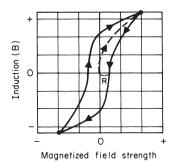
**Figure 9.3** Graph of the magnetic hysteresis loop resulting from magnetization and demagnetization of iron. The dashed line is a plot of the induction from the initial magnetization. The solid line shows a reversal of the field and a return to the initial magnetization value. *R* is the remaining magnetization (*remnance*) when the field is reduced to zero.
