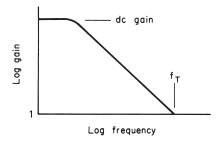
Figure 13.4 Amplitude-frequency response of a common-emitter or common-source amplifier.
