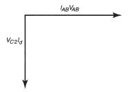
**Figure 16.8** Vector diagram of a reactance modulator producing FM. Note:  $V_g = V_{cz}$ . (From [1]. Used with permission.)
