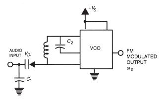
Figure 16.9 Voltage-controlled direct-FM modulator. (From [1]. Used with permission.)
