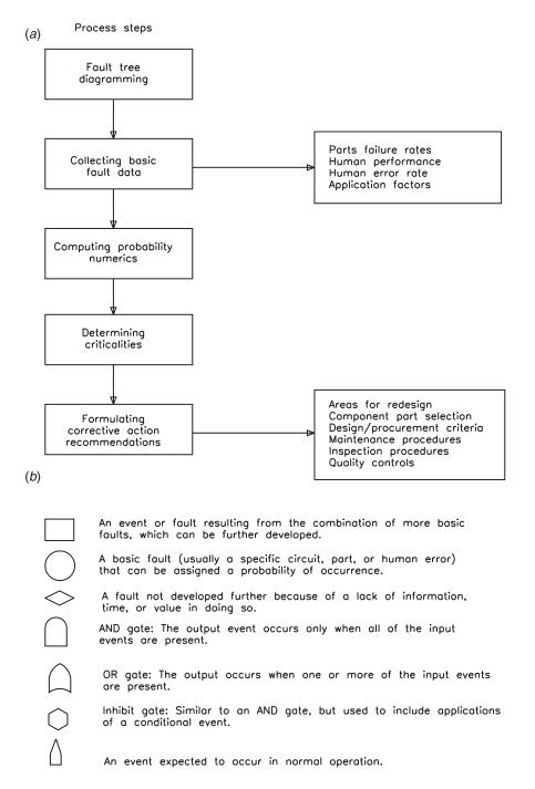
**Figure 20.1** Example fault tree analysis diagram: (a) process steps, (b) fault tree symbols, (c) example diagram (next page).
