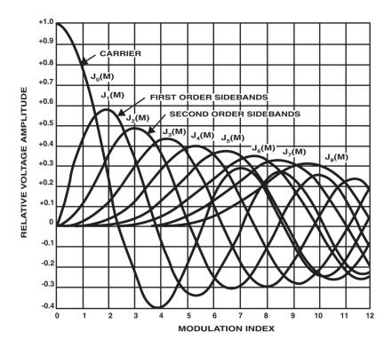
$\textbf{Figure 16.1} \ \ \text{Plot of Bessel functions of the first kind as a function of modulation index}.$
