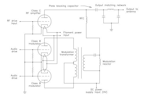
Figure 15.3 Simplified diagram of a high-level amplitude-modulated amplifier.
