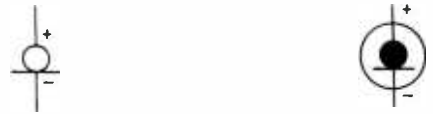
Fig. 14. Constant-current FET diodes are depicted in either of the two ways shown here. They are treated as diodes.
