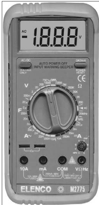
Figure 9-2: Multimeters measure voltages, resistance and current.
