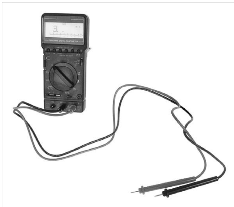
Figure 12-1: Multimeters measure voltage, resistance, current and continuity.
