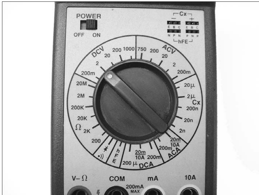
Figure 12-3: Digital multimeters provide a wide variety of measurement options.
