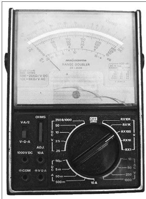
Figure 12-2: An analogue multimeter uses a needle to indicate voltage, current and other values, but we suggest you start with a digital model.
