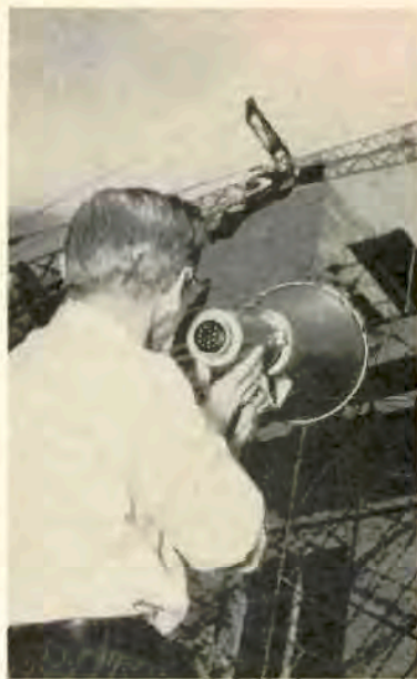
Fig. 6. With the transistor reducing space requirements of tubes and batteries, an electronic megaphone can contain microphone, amplifier, batteries and speaker in one independent unit. (Courtesy General Electric Co.)
