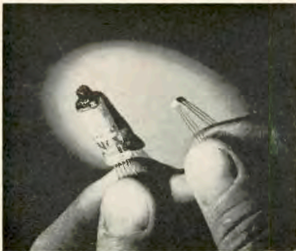
Fig. 5. The junction transistor is tiny compared to the "sub-miniature" tube, the smallest type made. These are approximately full size. (Courtesy General Electric Co.)
