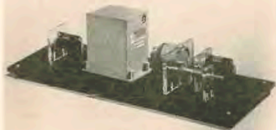
Fig. 8. This "servo" magnetic amplifier may be used to drive a mechanical positioning system. (Courtesy Magnetic Amplifiers, Inc.)
