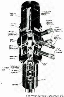
Fig. 5—Cutaway of a typical Klystron tube.
