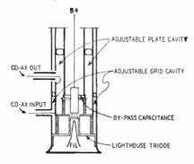
Fig. 2-Lighthouse tube in co-oxiol circuit.
