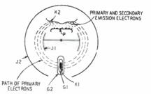
Fig. 3—Operation of the "orbital-beam" tube.
