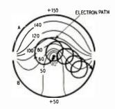
Fig. 6—Electrons in split-plate magnetron. RADIO-ELECTRONICS for
