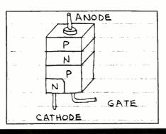
The physical construction and schematic symbol for the SCR are shown in (D). Frequently, single-letter designations are used to identify the leads: A for anode, K (or C) for cathode, and G for gate.
