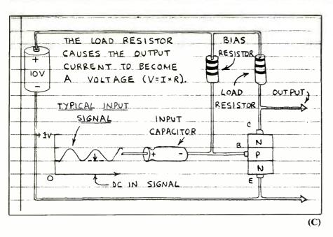
the bias resistor, only the positive half of the input signal *above* 0.6 volt will be amplified. This will cause severe distortion.
