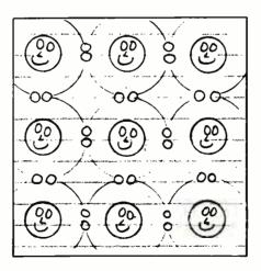
A cluster of silicon atoms sharing outer electrons forms a regular arrangement called a crystal. To keep things simple, in the above drawing of a silicon crystal, only the outer electrons are shown. Pure silicon isn't very useful. That's why silicon makers spice up their silicon recipes with a dash of phosphorous, boron, or other goodies. This is called "doping" the silicon. Then silicon has very useful electrical properties indeed!
