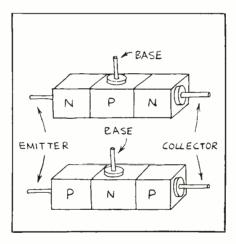
ing through the other two leads. This means transistors can be used as amplifiers and switches. There are two main families of transistors: bipolar and field-effect. We will concentrate here only on bipolar transistors.
