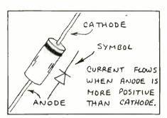
fies the *cathode* terminal. The opposite terminal is the anode. The above drawing illustrates both the physical packaging of the diode and its schematic symbol.
