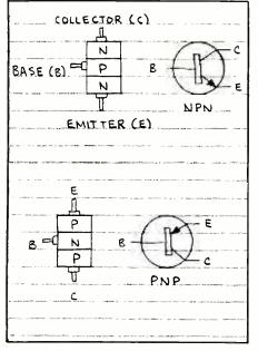
Note that the arrow in the emitter leads always points in the direction of hole flow. If the arrow points away from the base, the emitter is made of *n*-type material, which identifies it as an *npn* transistor. Conversely, if the arrow points toward the base, the base is *n*-type material, which means the emitter and collector are both *p*-type material and, thus, the transistor is a *pnp* device.
