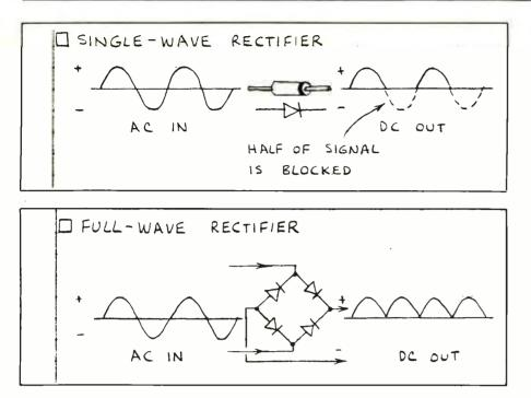
nations produce outputs in the fullwave circuit. This difference offers significant advantages, in the case of the full-wave circuit, when the output must be filtered to obtain a smooth (minimal-variation) dc voltage with minimum ripple.
