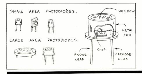
reverse-biased. A current flows when the *pn* junction is illuminated. When dark, a tiny current, called the "dark current," will flow.
