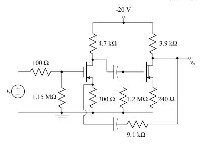
**8.29.** Determine the closed-loop gain, input resistance, and output resistance of the amplifier shown below. The NMOSFETs are identical with the following characteristic parameters:
