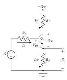
Figure 7.7: Common-collector power amplifier.
