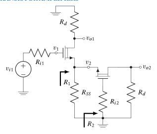
Figure 6.15: AC equivalent circuit for source-coupled pair (single input source).
