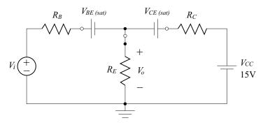
Figure 7.9: Re-drawn saturation model of the power amplifier in Figure 7.8c.
