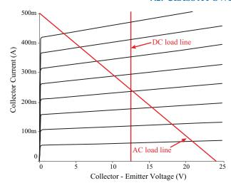
Figure 7.19: Output characteristics of the transformer-coupled Class A power amplifier shown in Figure 7.18.
