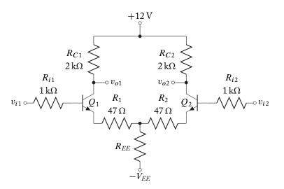
**6.21.** For the differential amplifier shown, find  $i_L$  in terms of the common- and differential-mode input signals. Assume identical transistors with  $\beta_F = 120$ .
