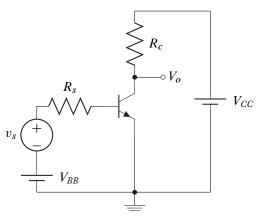
Figure 5.8: A simple common-emitter amplifier.
