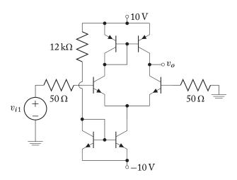
**6.29.** The differential amplifier shown uses identical BJTs. The BJT parameters are:
