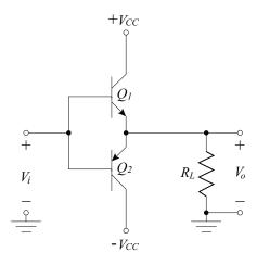
Figure 7.24: Simplified complementary Class B output stage.
