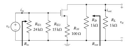
The AC equivalent circuit leads to the small-signal equivalent circuit for the amplifier:
