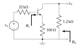
The voltage gain, as defined, is determined from Equation (5.59):
