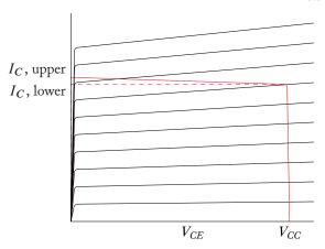
**Figure 6.27:** The characteristic curve of the active load device  $Q_1$  superimposed on the output characteristic curves for  $Q_3$ .
