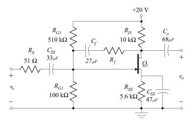
**8.20.** Complete the design of the circuit shown for a closed-loop gain  $A_{Vf} = -10$ . The JFET characteristic parameters are:
