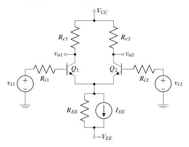
Figure 6.11: A typical emitter-coupled pair circuit diagram.
