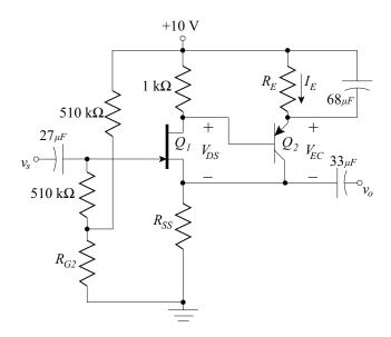
**8.33.** For the differential amplifier shown, find the closed-loop gain, input resistance, and output resistance of the amplifier. Assume identical transistors with  $\beta_F = 120$ . Use SPICE to confirm closed-loop gain of the amplifier.
