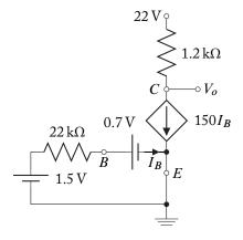
Both currents are positive: only  $V_{CE}$  must be checked to see if it is larger than  $V_{CE(sat)} = 0.2 \text{ V}$ . Kirchhoff's Current Law applied to the collector-emitter loop yields:
