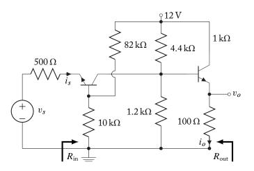
**6.3.** The amplifier shown uses identical transistors with the following characteristics:
