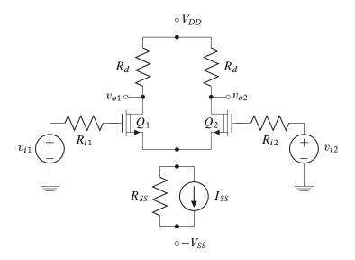
Figure 6.13: A typical source-coupled pair circuit diagram.
