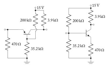
**6.6.** In most multistage amplifier designs, common-collector amplifier stages are best used as output stages to an amplifier cascade: they have little value when used as input or intermediate stages. Investigate this simple design principle by comparing the voltage and current gain of two-stage, capacitively-coupled cascades consisting of the two given amplifiers in the two configurations: CC-CE and CE-CC.
