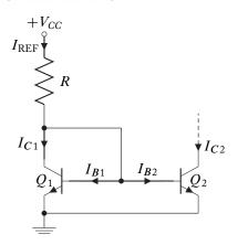
Figure 6.18: The simple BJT current mirror.
