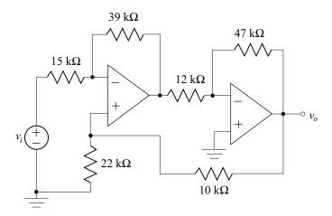
**8.38.** The characteristics of the amplifier shown include high input resistance with moderate voltage gain and output resistance. It is desired to reduce the output resistance of the amplifier through the use of feedback without significantly altering the input resistance.
