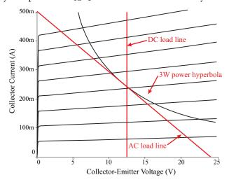
The quiescent base current is approximately  $I_B = 1.1 \,\mathrm{mA}$ . Also drawn on the load line graph is the 3W constant power dissipation hyperbola. A rough calculation may be made to determine the base bias resistor  $R_{BB}$ . Assuming that  $V_{BB} = V_{CC}$ ,
