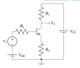
Figure 5.11: A common-emitter amplifier with an emitter resistor.
