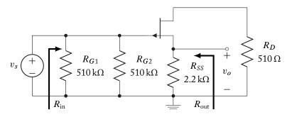
The small-signal models for *p*- and *n*-channel devices are identical and are based on the Q-points determined by the external circuitry. The AC equivalent circuit leads to the small-signal equivalent circuit for the *p*-channel JFET common-drain amplifier:
