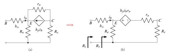
Figure 5.13: AC equivalent circuits—non-zero  $h_{oe}$ .
