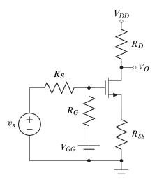
Figure 5.30: A common-source amplifier with source resistor.
