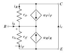
The small-signal ratios can be obtained by applying Kirchhoff's current law applied at the base node:
