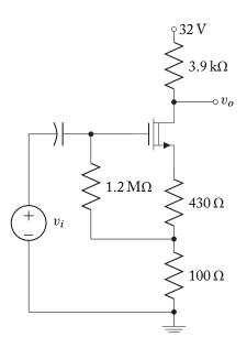
**5.33.** The common-emitter amplifier with constant current source biasing shown does not meet the required design specifications. The specifications are:
