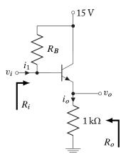
**5.9.** Complete the design by finding the value for  $R_B$  so that the quiescent  $I_C = 2 \text{ mA}$ . Determine the quiescent voltages and currents. Draw the midband small-signal equivalent circuit for the circuit below, and determine the midband input resistance  $R_{in}$ , output resistance  $R_{out}$ , and voltage gain of the circuit.
