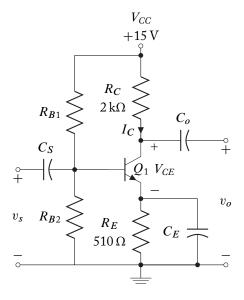
**5.40.** Complete the design of the circuit shown for maximum symmetrical swing in the midband frequency range. The circuit is required to be have a bias stability of 1% change in  $I_C$  for a 10% change in  $\beta_F$ . The pnp BJT has a  $\beta_F = 120$  and  $V_A = 120$  V.
