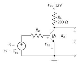
Figure 7.2: Common-emitter power amplifier.
