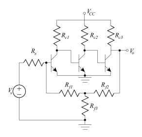
**8.18.** For the single stage amplifier shown, determine the value of  $R_f$  to achieve an overall midband voltage gain of magnitude 8.
