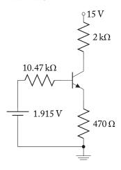
Now that the forward-active region is verified, the BJT *b*-parameters can be determined:
