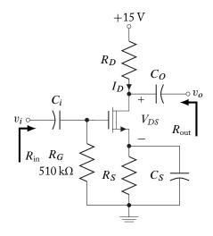
**5.24.** The MOSFET amplifier circuit shown is to be designed for a midband voltage gain of -8. The circuit is to be biased for the following quiescent condition:
