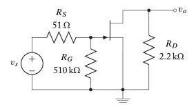
Step #4 Determine the AC performance by replacing the FET by its AC model. The small-signal circuit model of the amplifier is shown below.
