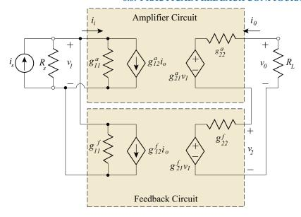
Figure 8.10: Two-port realization of a shunt-series feedback amplifier.
