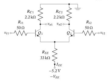
**6.31.** In order to boost the input resistance of a differential amplifier, resistors are often added between the emitters of the emitter-coupled BJT pair. For the circuit shown calculate the differential voltage gain, input resistance, and the CMRR. Compare appropriate results with a circuit without these emitter resistors (Examples 6.4 and 6.5).
