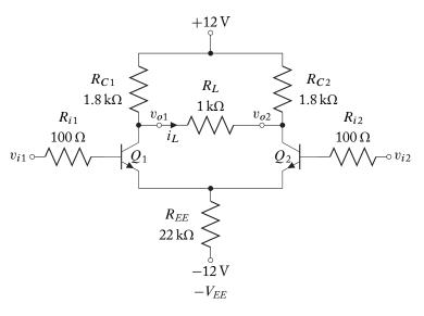
**6.22.** The transistors in the differential amplifier shown below are identical and have the following characteristics:
