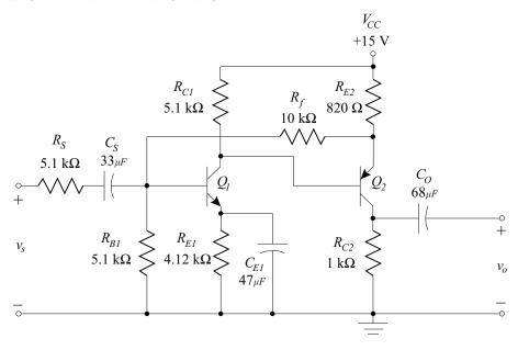
**8.24.** Determine the closed-loop gain, input resistance, and output resistance of the amplifier shown below. The transistors are identical and have the following characteristic parameters:
