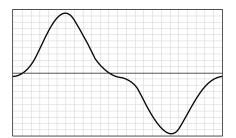
**7.29.** Amplifiers may distort the input signal in rather unusual ways. For instance a Class A, common-emitter amplifier with an emitter resistor responds to an overly-large input as show.
