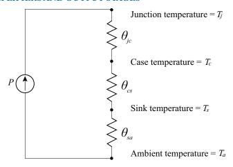
Figure 7.34: Heat transfer model.
