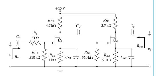
**6.9.** For the circuit shown, the transistor parameters are:
