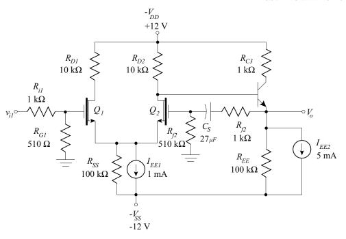
8.35. The series-shunt feedback amplifier of Example 8.5 is to be redesigned to have larger voltage gain. This change is to be accomplished by alteration of the feedback (1.2 k $\Omega$ ) resistor *only*. If the requirement on the midband input resistance,  $R_{in}$ , is reduced to:
