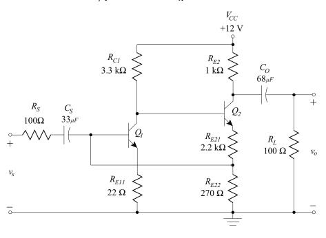
**8.25.** Determine the closed-loop gain, input resistance (not including the source resistor,  $R_S$ ), and output resistance of the amplifier shown below. The transistors are identical and have the following characteristics:
