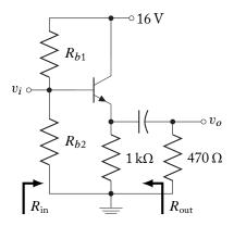
5.37. Complete the design of the circuit shown for maximum symmetrical collector current swing. Let  $\beta_F = 180$ ,  $V_{\gamma} = 0.7 \,\mathrm{V}$ , use the "rule of thumb" relationship between  $R_E$ and  $R_B$  for stable operation (1% change in  $I_C$  for 10% change in  $\beta_F$ ). Determine the quiescent conditions.
