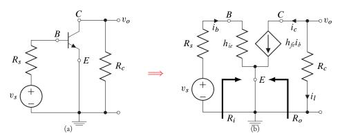
**Figure 5.9:** AC modelling of a simple common-emitter amplifier. (a) The small-signal circuit: DC sources set to zero; (b) BJT replaced by *h*-parameter model.
