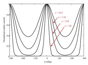
Figure 7.6: Normalized emitter current vs. angle for varying base-emitter voltages.
