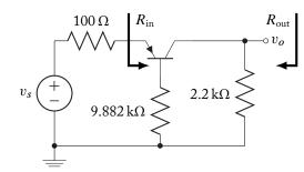
$$R_{in} = \frac{h_{ie} + R_b}{h_{fe} + 1} = \frac{410 + 9191}{121} = 71.1 \,\Omega$$
