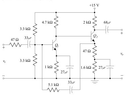
**8.27.** The shunt-series feedback amplifier of Example 8.4 is to be redesigned to have a voltage gain:
