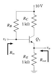
**5.10.** Draw the midband small-signal equivalent circuit for the circuit below. Find the expressions for the midband input resistance  $R_{in}$ , output resistance  $R_{out}$ , and voltage gain of the circuit.
