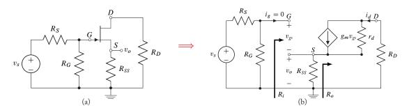
**Figure 5.35:** AC modeling of a common-drain amplifier. (a) The small-signal circuit: DC sources set to zero. (b) FET replaced by the small-signal model.
