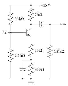
A SPICE simulation of the maximum symmetrical swing properties of both  $V_{CE}$  and  $v_o$ for this circuit follows. The rounding of resistor values and the fact that the simulation value of  $V_{CE(sat)} = 0.05 \,\mathrm{V}$  rather than 0.2 V as used in calculations has introduced a slight deviation in both the Q-point and the swing. Distortion is the cause of dissimilar shaped limiting of the signal at the two ends.
