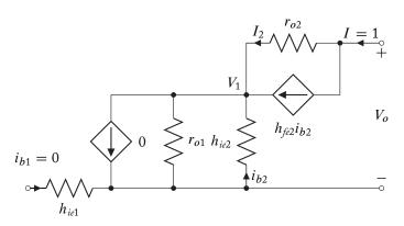
**Figure 6.9:** Equivalent circuit for calculation of cascode  $h_{oe}$ .
