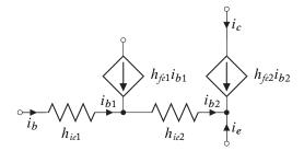
Figure 6.7: The AC model for a common-collector—common emitter Darlington pair.
