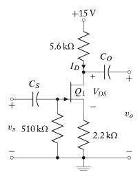
**5.23.** Complete the design of the *n*-channel depletion MOSFET circuit to achieve a Qpoint:  $I_D = 1 \text{ mA}$ , and  $V_{DS} = 4 \text{ V}$ .
