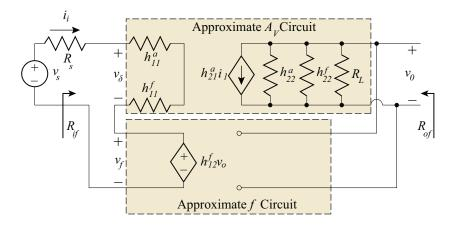
Figure 8.13: Redistributed series-shunt realization.
