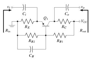
**5.11.** Complete the design of the circuit below for  $R_{in} = 1.5 \,\mathrm{k}\Omega$  and determine the quiescent currents and voltages. Draw the midband small signal equivalent circuit. Determine the appropriate *b*-parameters for the small signal model and find the midband voltage gain, input resistance  $R_{in}$ , and output resistance  $R_{out}$ . Assume that
