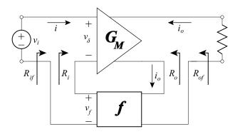
Figure 8.5: Input and output resistance for series-series feedback.
