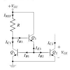
Figure 6.19: Three transistor current mirror.
