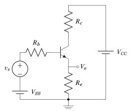
Figure 5.15: A typical common-collector amplifier.
