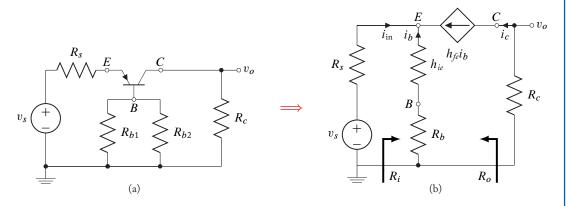
Figure 5.21: AC modeling of a common-base amplifier. (a) The small-signal circuit: DC sources set to zero. (b) BJT replaced by h-parameter model.
