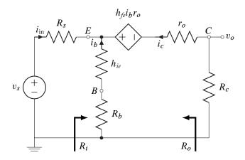
**Figure 5.22:** Common-base amplifier AC equivalent circuit including  $r_o$ .
