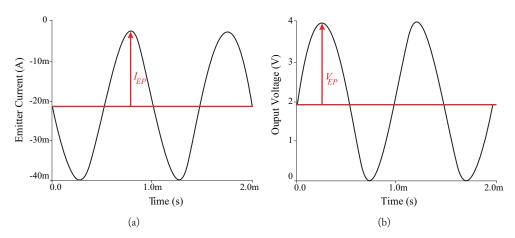
**Figure 7.11:** Peak values of the (a) emitter current and (b) emitter (load) voltage derived from the current and voltage waveforms.
