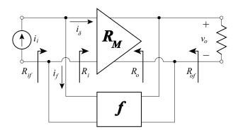
Figure 8.4: Input and output resistance for shunt-shunt feedback.
