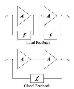
**8.12.** Complex amplifiers may incorporate both local and global feedback. The amplifier shown is an example of such a complex amplifier. Derive the transfer characteristic for this amplifier.
