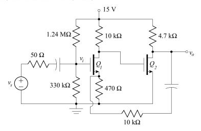
This amplifier is known to have the to have high input resistance ( $\approx 260 \, k\Omega$ ), moderate output resistance ( $\approx 300 \, \Omega$ ), and a midband voltage gain:
