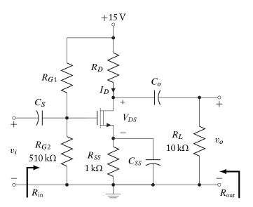
**5.26.** Complete the design of the amplifier shown to establish operation at  $V_{GS} = V_{DS} = 2V_T$  with equal values of  $R_S$  and  $R_D$ . The input resistance,  $R_{in}$ , is 730 k $\Omega$  ± 5%. The *n*-channel enhancement MOSFET parameters are:
