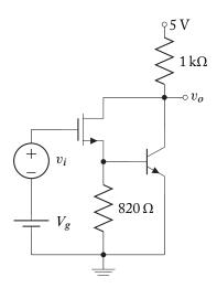
**6.16.** Determine the quiescent currents and voltages, and the midband voltage gain of the Darlington common-base amplifier shown below. Identical transistors are used with parameters:
