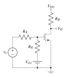
Figure 5.27: A simple common-source amplifier.
