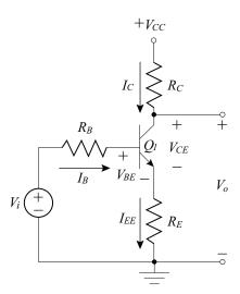
Figure 7.14: Common-emitter power amplifier.
