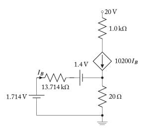
The collector-emitter voltage must be checked to make sure the composite transistor is in the forward active region:
