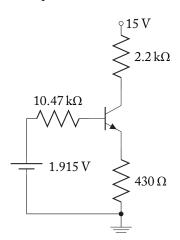
The base and collector currents are calculated to be:
