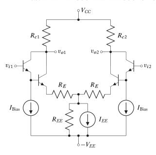
Figure 6.16: Simplified input stage schematic: LM318 OpAmp.
