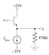
7.3. A power amplifier to drive a load,  $R_L = 220 \,\Omega$ , with the basic topology shown is under design. The Silicon power BJT is described by:
