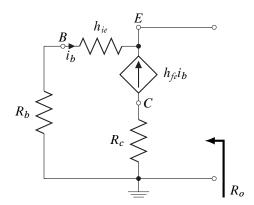
Figure 5.17: Common-collector output resistance AC equivalent circuit.
