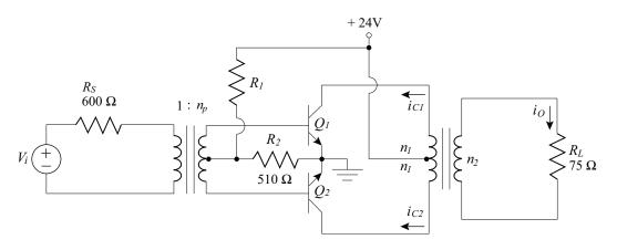
**7.20.** Complete the design of a direct-coupled output push-pull amplifier, shown to achieve a maximum output to an 8  $\Omega$  load. The circuit uses matched transistors with the following specifications:
