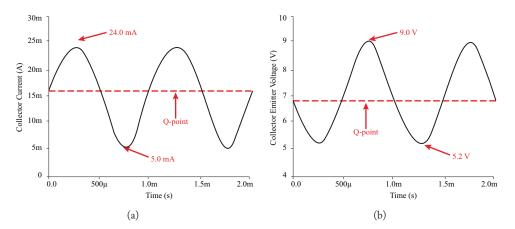
Figure 7.5: Output voltage and current waveforms for the power amplifier of Figure 7.2: (a) collector current; and (b) collector-emitter voltage.
