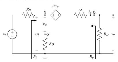
**Figure 5.40:** Alternate small-signal model of the common-gate amplifier using the small-signal model of the FET with voltage-controlled voltage source.
