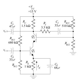
**8.31.** The amplifier shown is to be used as the basis for a series-shunt feedback amplifier with a voltage gain of twelve (12). The JFETs are described by:
