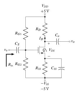
**5.27.** Complete the design of the common-gate amplifier so that  $I_D = -1$  mA. Determine the quiescent voltages and currents, the voltage gain,  $A_{vs} = \frac{v_o}{v_s}$ ,  $R_{in}$ , and  $R_{out}$ .
