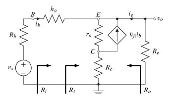
Figure 5.18: AC equivalent circuit—common-collector amplifier.
