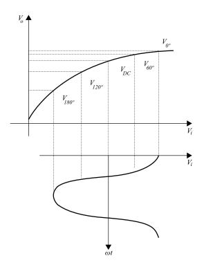
Figure 7.32: Graphical determination of the distortion content in the output voltage.
