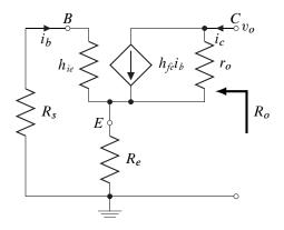
Figure 5.14: Circuit for calculation of output resistance.
