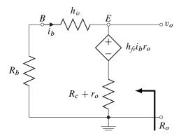
Figure 5.19: AC equivalent circuit for output resistance calculation.
