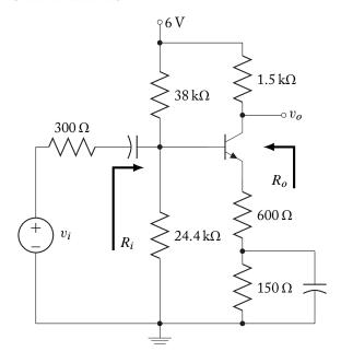
5.7. Complete the design by finding the value for  $R_E$  to establish the given quiescent conditions. Draw the midband small signal equivalent circuit for the circuit below. Determine the appropriate b-parameters for the model and find midband input resistance  $R_{in}$ , output resistance  $R_{out}$ , and voltage gain of the circuit.
