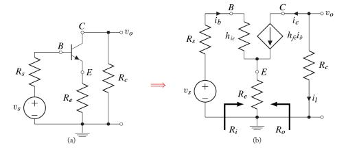
Figure 5.12: AC modeling of a common-emitter amplifier with an emitter resistor. (a) The smallsignal circuit: DC sources set to zero; (b) BJT replaced by h-parameter model.
