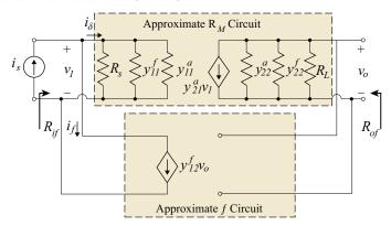
Figure 8.9: Redistributed shunt-shunt realization.
