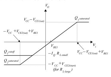
Figure 7.13: Transfer characteristic of the common-collector power amplifier of Figure 7.12.
