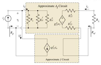
Figure 8.11: Redistributed shunt-series realization.
