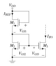
Figure 6.24: Simple enhancement NMOSFET current mirror.
