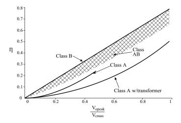
**Figure 7.29:** Typical conversion efficiency of well-designed power amplifiers as a function of output signal amplitude.
