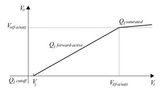
Figure 7.10: Transfer characteristic of the common-collector power amplifier in Figure 7.7.
