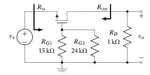
The AC equivalent circuit leads to the small-signal equivalent circuit for the common-gate amplifier:
