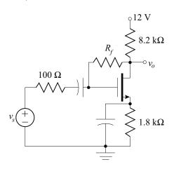
8.19. Complete the design of the circuit shown to achieve a closed-loop gain
