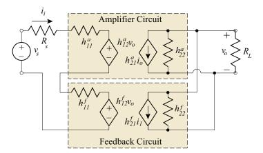
Figure 8.12: Two-port realization of a series-shunt feedback amplifier.
