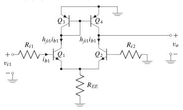
Figure 6.36: AC model of the emitter coupled differential amplifier in Figure 6.35.
