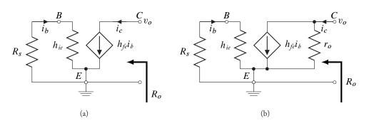
**Figure 5.10:** Circuit for calculation of output resistance. (a) Small-signal output circuit: AC source set to zero; (b) More accurate BJT *h*-parameter model.
