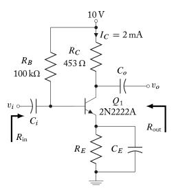
**5.8.** For the common-collector circuit shown, assume a Silicon BJT with  $\beta_F = 75$ .
