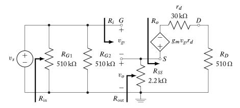
The voltage gain of the amplifier is,
