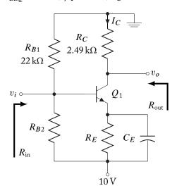
**5.12.** Complete the design of the circuit below and draw the midband small signal equivalent circuit. Determine the quiescent currents and voltages. Draw the small signal equivalent circuit. Determine the appropriate b-parameters for the small signal model and find the midband voltage gain, input resistance  $R_{in}$ , and output resistance  $R_{out}$ .
