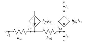
Figure 6.5: The AC model for a dual common-collector Darlington pair.
