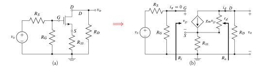
**Figure 5.31:** AC modeling of a common-source amplifier with a source resistor. (a) The small-signal circuit: DC sources set to zero. (b) The FET replaced by the small-signal model.
