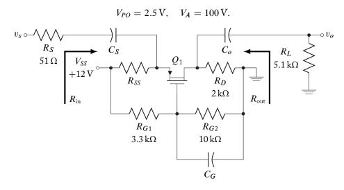
**5.28.** Design a non-inverting amplifier with midband voltage gain  $A_{vs} \ge 2$  and output resistance,  $R_{out}=1\,\mathrm{k}\Omega\pm20\%$ , input resistance,  $R_{in}=100\,\Omega\pm25\,\Omega$  using the 2N5461 pchannel JFET. The 2N5461 specification sheet is found in the appendix. Use the typical
