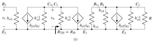
**Figure 6.29:** (a) AC and (b) Small-signal of the common-emitter amplifier with active load in Figure 6.26.
