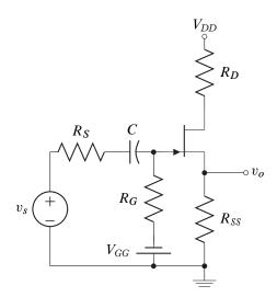
Figure 5.34: A simple common-drain amplifier.
