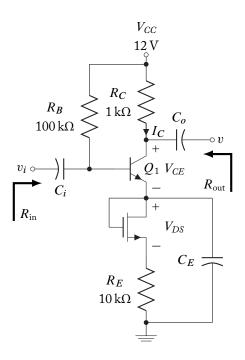
**5.34.** The common-collector buffer amplifier (using  $Q_1$ ) shown does not meet the required design specifications. The FET  $Q_2$  forms a constant current source. The specifications are:  $I_C = 2 \text{ mA}$ ,  $Q_1$  maximum DC power dissipation:  $15 \text{ mW}(P_D = I_C, V_{CE} \le 15 \text{ mW})$ .
