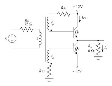
7.21. Design a Class B power amplifier stage to deliver an average power of 75 W into a  $12\,\Omega$  load. The power supply must be 5 volts greater than the peak sinusoidal output signal.
