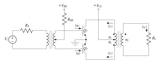
Figure 7.33: Class B push-pull arrangement.
