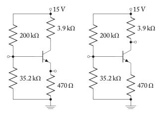
**6.7.** In most multistage amplifier designs, common-gate amplifier stages are best used as input stages to an amplifier cascade: they have little value when used as intermediate or final stages. Investigate this simple design principle by comparing the voltage and current gain of two-stage, capacitively-coupled cascades consisting of the two given amplifiers in the two configurations: CG-CS and CS-CG.
