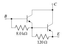
In AC analysis the resistors slightly decrease the effective value of the two dominant h-parameters,  $h_{ie}$  and  $h_{fe}$ , in each BJT. For this Darlington pair assume each individual BJT in the typical circuit diagram is described by  $\beta_F = 60$ .
