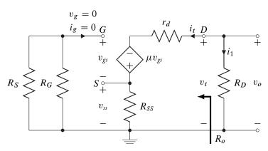
Figure 5.33: Circuit for calculating the output resistance of the common-source amplifier with source resistor.
