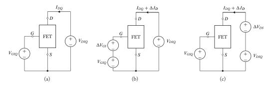
**Figure 5.23:** (a) Generic FET biased in the saturation region by a gate-source voltage  $V_{GSQ}$ , with a drain-source voltage  $V_{DSQ}$  and drain current  $I_{DQ}$ . (b) Method for determining gate small-signal transconductance with small variations in  $V_{GS}$  causing small changes in  $I_D$ . (c) Method for determining drain small-signal conductance with small variations in  $V_{DS}$  causing small changes in  $I_D$ .
