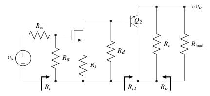
The total input resistance,  $R_i$ , is the parallel combination of  $R_g$  and the input resistance of the common-source stage:
