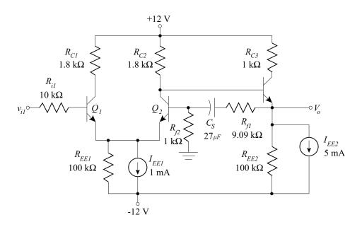
**8.34.** The transistors in the differential amplifier shown are identical and have the following characteristics:
