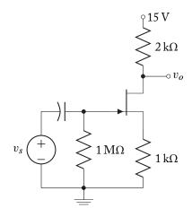
**5.22.** Find the midband voltage gain for the circuit shown. The *n*-channel JFET parameters are:
