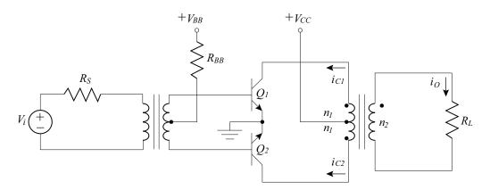
Figure 7.20: Class B common-emitter push-pull power amplifier.
