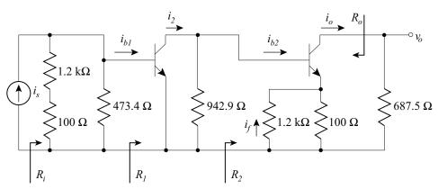
In addition, the feedback ratio, f, is easily determined from the output loading circuit. The feedback current is identified in the output circuit (feedback current is *subtracted* from the input, thus it flows *toward* the output port) and a ratio is formed:
