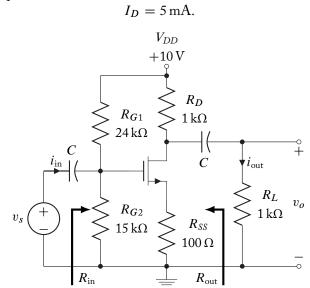
Determine the following circuit parameters:
