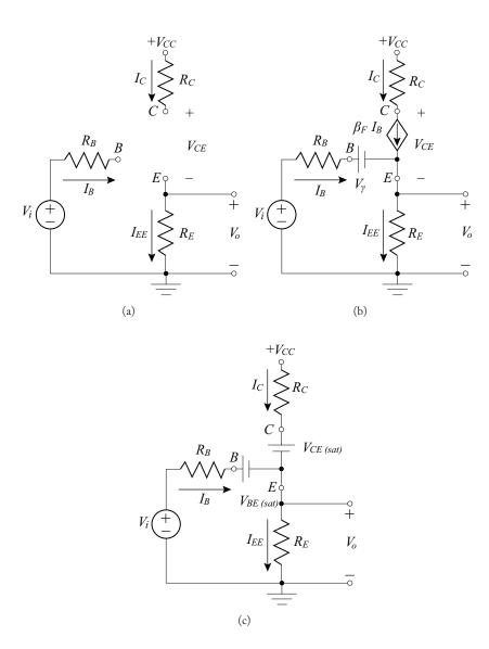
Figure 7.8: Equivalent models for the (a) cutoff, (b) forward-active, and (c) saturation regions for the common-emitter power amplifier in Figure 7.7.
