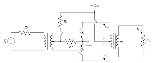
Figure 7.26: Class AB power amplifier configuration.
