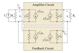
Figure 8.8: Two-port realization of a shunt-shunt feedback amplifier.
