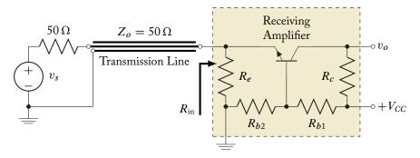
The expressions for the input resistance and voltage gain of a common-base amplifier are found in Table 5.5:
