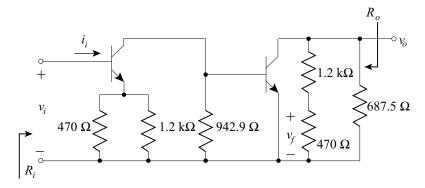
In addition, the feedback ratio, f, is easily determined from the output loading circuit. The feedback voltage is identified on the output loading circuit (feedback voltage is subtracted from the input, thus its positive pole is toward the output port) and a ratio is formed:
