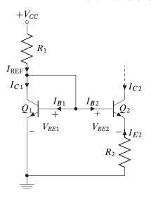
Figure 6.21: The Widlar current source.
