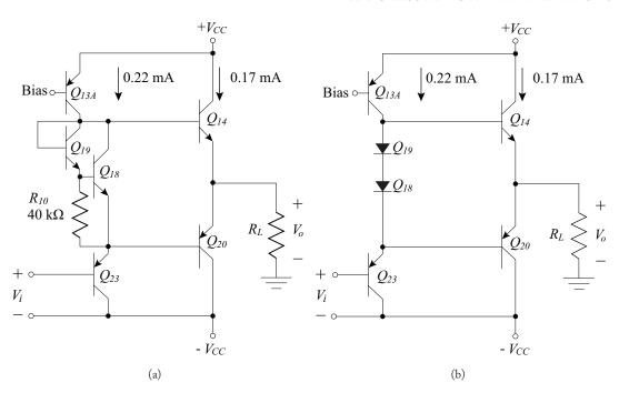
Figure 7.28:  $\mu$  A741 OpAmp output stage (a) Actual schematic; (b) Simplified schematic.
