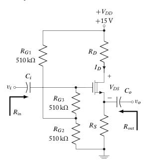
**5.32.** Assume an *n*-channel depletion type MOSFET with parameters:
