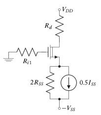
Figure 6.14: A half-circuit equivalent for quiescent condition calculation.
