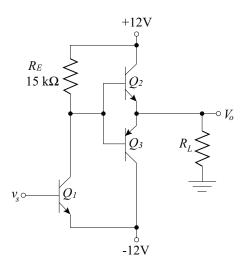
7.14. The common-drain class B amplifier shown uses devices for which
