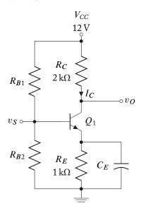
**5.38.** Design an inverting amplifier with a gain of  $35 < |A_v| < 45$  with an input resistance of  $12 \,\mathrm{k}\Omega \pm 20\%$  and an output resistance of  $3.5 \,\mathrm{k}\Omega \pm 20\%$ . Use a 2N2222 BJT and design for maximum symmetrical swing. Available power supply voltages:  $+15 \,\mathrm{V}$ .
