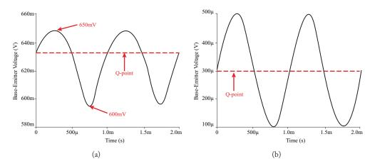
Figure 7.4: Input voltage and current waveforms for the power amplifier of Figure 7.2: (a) The baseemitter voltage; (b) base current (pure sinusoid).
