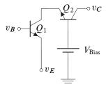
**Figure 6.8:** The cascode configuration.
