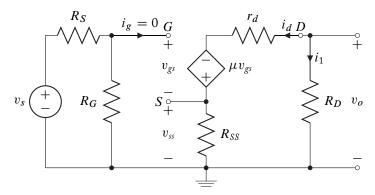
**Figure 5.32:** Alternate small-signal model of the common-source amplifier with source resistor using the small-signal model of the FET with voltage-controlled voltage source.
