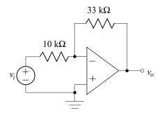
**8.22.** Use the principles of feedback analysis to find the closed-loop voltage gain, the input resistance  $R'_{if}$ , and output resistance  $R'_{of}$ . The OpAmp open-loop gain is  $A_V = 10 \,\mathrm{kV/V}$ , input resistance of the OpAmp is 1 M $\Omega$ , and the output resistance of the OpAmp is 75  $\Omega$ .
