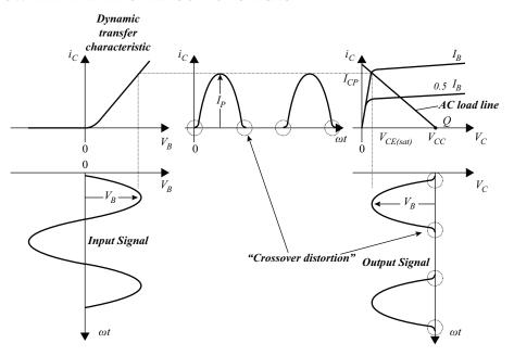
**Figure 7.21:** Waveforms of a single class B transistor stage (half of a push-pull stage) constructed with graphical methods.
