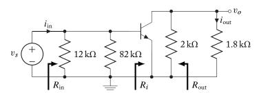
$$A_{V} = -\frac{h_{fe}R_{c}}{h_{ie}} = -\frac{150(2 \text{ k}//1.8 \text{ k})}{1.755 \text{ k}} = -81.0$$
