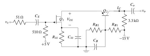
**6.15.** For the BiFET Darlington configuration shown, the bias voltage  $V_g$  is adjusted so that the quiescent output voltage is 2.5 V. The transistor parameters are as follows:
