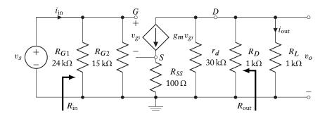
$$A_{VS} = A_{V} = -\frac{g_{m}r_{d}R_{D}}{R_{SS} + r_{d} + R_{D} + g_{m}r_{d}R_{SS}}$$
