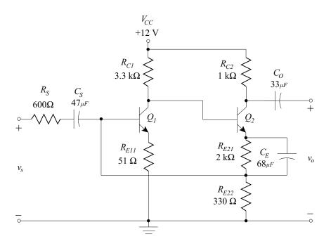
**8.26.** Determine the closed-loop gain, input resistance (not including the source resistor,  $R_S$ ), and output resistance of the amplifier shown below. The transistors are identical and have the following characteristic parameters:
