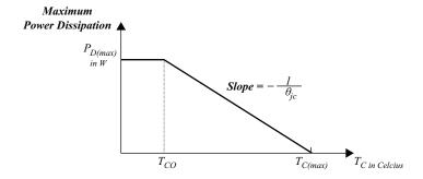
**Figure 7.35:** Transistor power dissipation derating curve.
