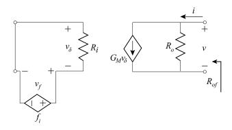
Figure 8.7: Schematic representation of series-series feedback for output resistance calculations.
