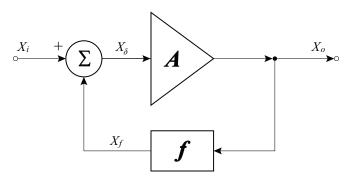
Figure 8.1: Basic negative feedback topology.
