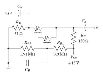
**6.17.** For the circuit shown, the transistors parameters are:
