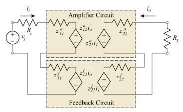
Figure 8.14: Two-port realization of a series-series feedback amplifier.
