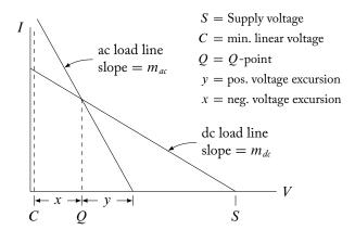
Figure 5.43: Typical amplifier AC and DC load lines.
