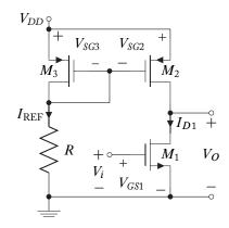
Figure 6.31: Common source amplifier with active load.
