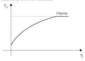
Figure 7.31: Non-linear transfer characteristic of a power amplifier.
