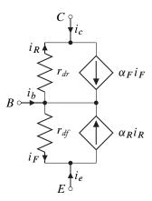
**Figure 5.5:** A forward-active small-signal model of a BJT.
