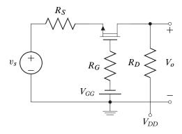
Figure 5.38: A simple common-gate amplifier.
