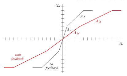
Figure 8.2: The effect on feedback on an amplifier transfer characteristic.
