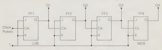
Fig. 9.15 The RIPPLE or ASYNCHRONOUS COUNTER.
