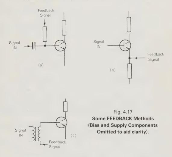
(a) Shunt Feedback into the Base. (b) Series Feedback into the Emitter.(c) Series Feedback using a Transformer.
