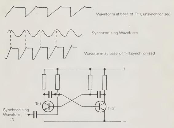
Fig. 7.17 A SYNCHRONISED MULTIVIBRATOR.
