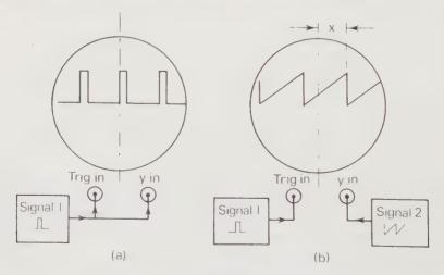
Fig. 1.9 Using an EXTERNAL TRIGGER to measure a Time Difference.
