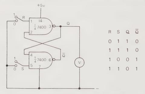
Fig. 9.9 The R-S FLIP-FLOP and its Truth Table.
