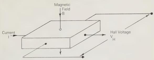
Fig 3.21 Schematic Diagram of a Hall-Effect Device.
