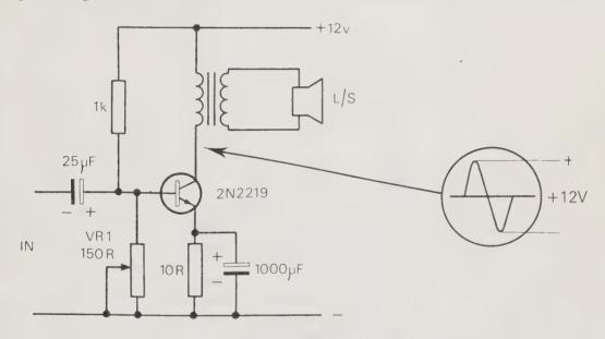
Fig. 5.4 A single-transistor CLASS A AMPLIFIER.
