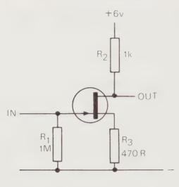
Fig. 4.9 BIASING CIRCUIT for a Junction FET.
