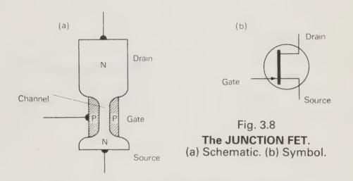
Look first at the structure of the junction FET (Fig. 3.8). A tiny bar of silicon of either type (the N-type is actually illustrated) has a junction formed near one end. Connections are made to each end of the bar, and also to the P-type material at the junction. The P-type connection is called the *gate*, the end of the bar nearest the gate the *source*, and the other end of the bar the *drain*.
