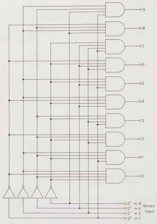
Fig. 9.19 A BINARY-TO-DECIMAL DECODER.
