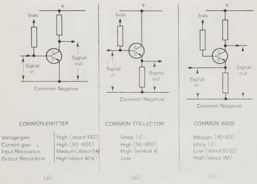
Fig. 3.7 The Three Circuit Connections of a Bipolar Transistor.
