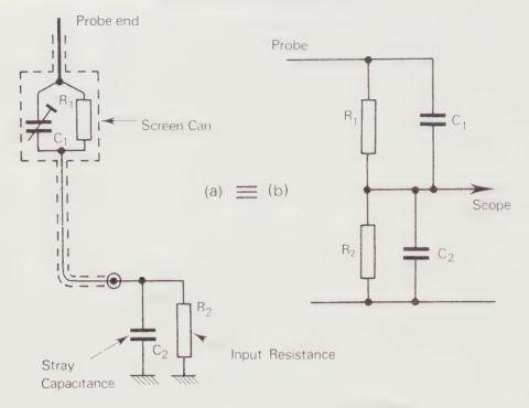
Fig. 1.10 A Low-Capacitance PROBE.
