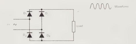
Fig. 2.11 FULL-WAVE BRIDGE RECTIFIER Circuit.
