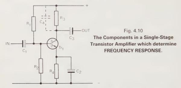
base of the transistor, and  $C_3$  prevents d.c. from its collector from affecting the next stage. The circuit can therefore give no voltage gain for d.c.; and the amount of gain it can give at low a.c. frequencies is inevitably limited by the action of the capacitors  $C_1$  and  $C_3$ . (Gain will also be affected by  $C_2$ , because this capacitor bypasses the negative feedback action of  $R_4$  for a.c. signals only).
