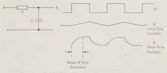
Fig. 7.19 The INTEGRATING Circuit, and Waveforms.
