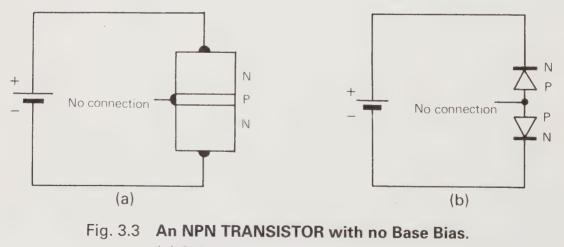
(a) Schematic. (b) Equivalent circuit.
