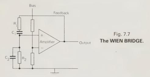
These RC circuits, also, require amplitude-stabilisation if they are to produce sine-waves of good quality, but they are capable of providing very low distortion figures (of the order of only 0.01%) by good design. An example of a Wien bridge oscillator circuit with provision for amplitude stabilisation is shown in Fig. 7.8. The amplifier itself is a 741 IC.
