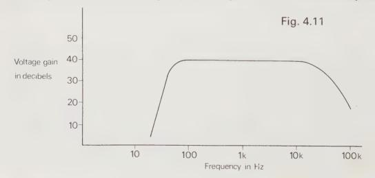
steps occupy equal lengths of horizontal scale. This type of scale is necessary to show the full frequency range of an amplifier.
