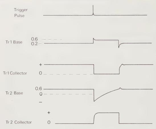
Fig. 7.14 Monostable Waveforms.
