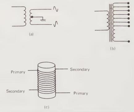
Fig. 8.3 Types of TRANSFORMER WINDINGS.
