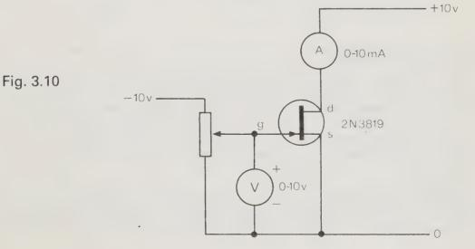
For the bias voltages listed, fill in the readings of current. Find also the *cut-off voltage*, which is the gate voltage at which channel current flow just reaches zero.
