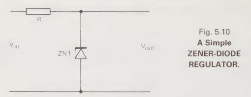
Voltage  $\times$  Maximum Current — with dissipation in milliwatts if the current is measured in mA.
