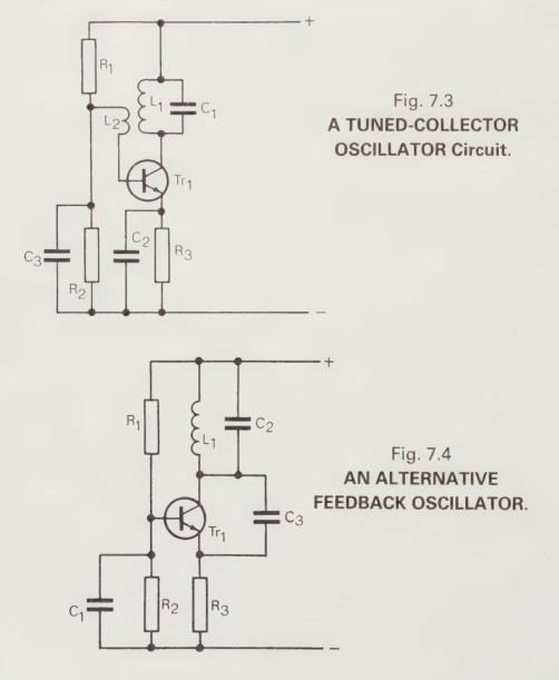
Remember that the output of a single-transistor common-emitter amplifier is always phase-inverted, so that another inversion must be carried out if feedback is to be taken from the collector to the base.
