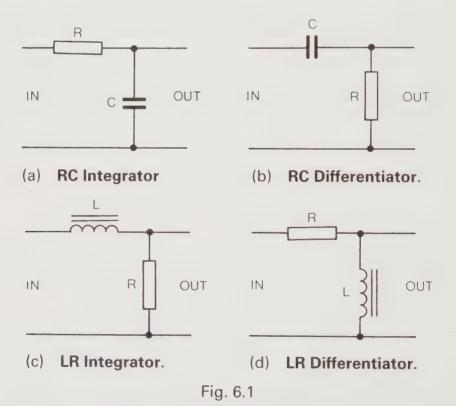
Some Circuits in which TRANSIENT CURRENTS can Flow.
