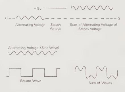
Fig. 1.15 WAVEFORM ADDITION.
