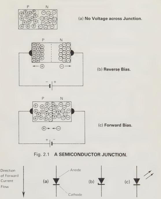
Fig. 2.2 DIODE SYMBOLS. (a) Signal or Rectifier Diode. (b) Zener Diode. (c) Light-emitting Diode (LED).
