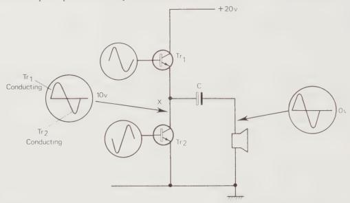
Fig. 5.5 A single-ended PUSH-PULL, or "TOTEM-POLE" circuit.
