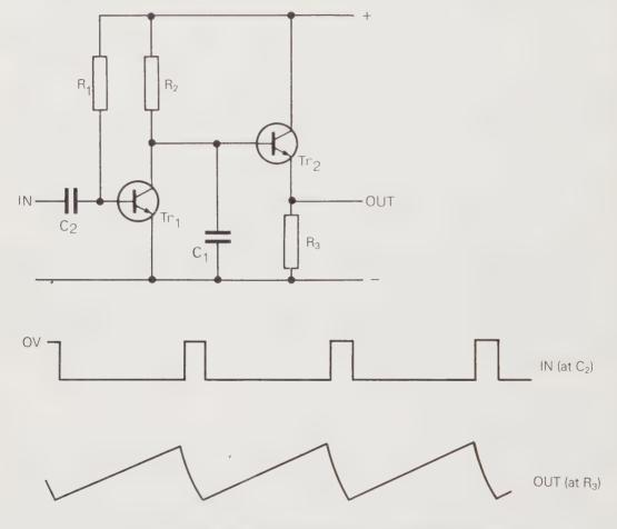
Fig. 7.20 A Simple TIMEBASE, or SWEEP, Circuit.
