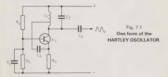
The amplitude of the oscillation is limited at the emitter, because the transistor will cut off if emitter voltage rises to a value more than about 0.5V below base voltage. The distortion of the wave-shape caused by this limiting effect is smoothed out by the "flywheel" effect of the tuned (or "tank") circuit  $L_1 C_2$ , which produces a sine-wave voltage at the resonant frequency even when the current waveform is not a perfect sine-wave.
