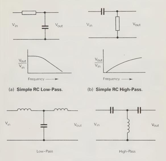
(c) More advanced LC Filters. Fig. 6.11 FILTERS.
