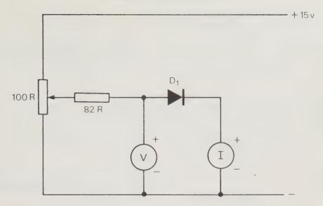
Fig. 2.3 Circuit for Measuring CURRENT THROUGH DIODE and VOLTAGE ACROSS DIODE.
