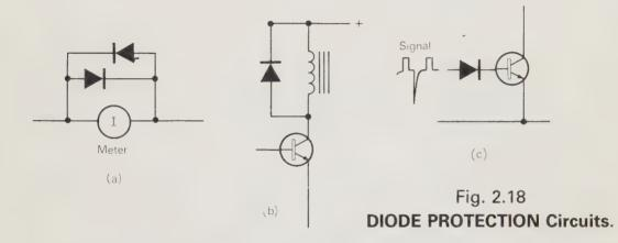
Fig. 2.18(b) shows the circuit of a diode used to protect a transistor which is switching current into an inductive load such as a relay. When the current across such a load is suddenly switched off, the voltage across the load rises to a very high value (many times the supply voltage), which can damage the transistor. A diode connected as shown will conduct when the voltage surge occurs, so protecting the transistor.
