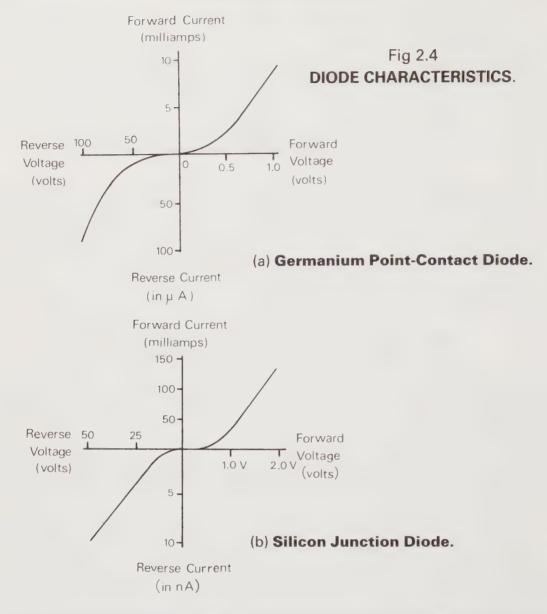
2. The reverse (leakage) current of a germanium diode is much greater than that of a silicon diode, being measured in  $\mu A$  whereas the silicon is measured in the much smaller nanoampere ( $1nA = 1/1000\mu A$ ).
