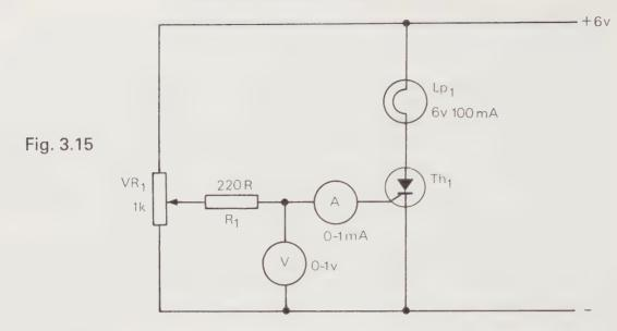
Thyristors are used for power control, using either a.c. or an unsmoothed rectified supply. By being made to fire at different parts of the cycle, the thyristor can be made to conduct for different percentages of the cycle, thus controlling average current flow through the load.
