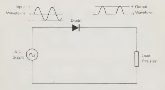
Fig. 2.7 A HALF-WAVE RECTIFIER Circuit.
