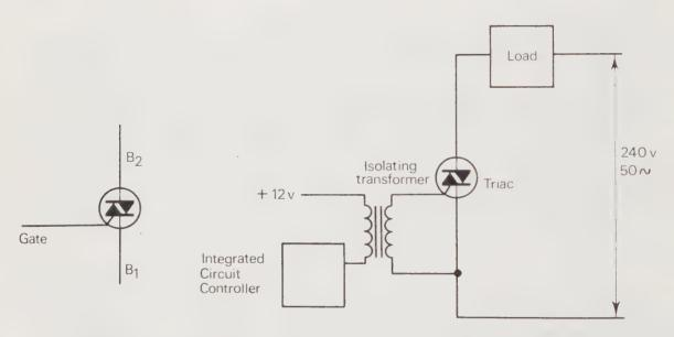
Fig. 3.18 The TRIAC. Symbol and Typical Connection.
