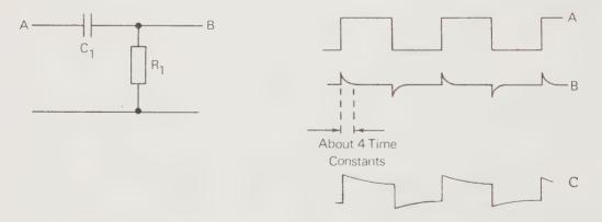
Fig. 7.18 The DIFFERENTIATING CIRCUIT, and Waveforms.
