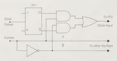
Fig. 9.17 The UP-DOWN COUNTER CONTROL.
