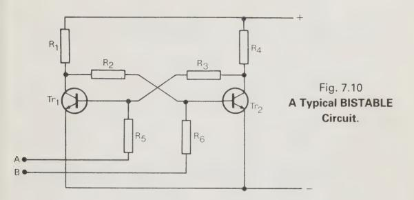
Fig. 7.10 shows a typical bistable circuit using two transistors. In one stable state, Tr1 is conducting with Tr2 cut off. In the other state, the conditions are reversed. Both states are stable.
