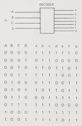
Fig. 9.21 Truth Table for a Binary Seven-Segment Decoder.
