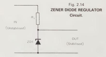
The complete circuit is therefore that shown in Fig. 2.14, with the output voltage across the diode being used to supply any other circuit or part of a circuit which requires a stable voltage. Many circuits, especially measuring and oscillator circuits, are adversely affected by voltage variation, which can be caused by changes in the supply voltage or by changes in the current drawn by the load.
