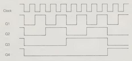
Fig. 9.16 BINARY COUNTER WAVEFORMS.
