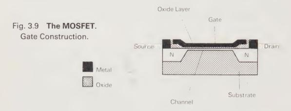
A positive voltage applied to the gate has the effect of attracting more electrons into the channel, and so increasing its conductivity. A negative potential so applied would repel electrons from the channel and so *reduce* its conductivity.
