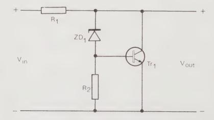
Fig. 5.11 The "AMPLIFIED-ZENER" REGULATOR Circuit.
