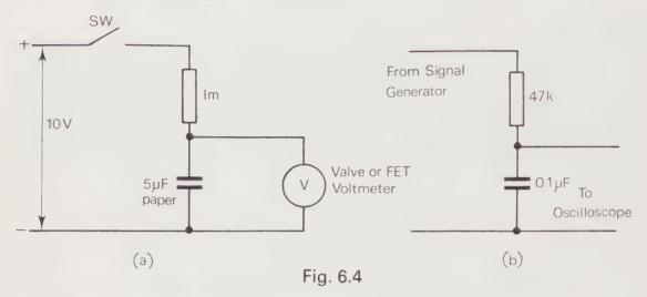
The reason for the shape of the graph obtained in *Exercise* 6.3 is that the voltage across the capacitor plates cannot change instantly when the voltage across the whole circuit is changed.
