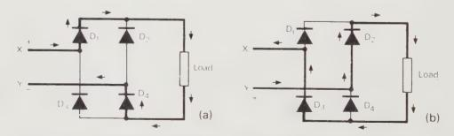
Fig. 2.12 CURRENT PATHS in the Bridge Rectifier Circuit.
