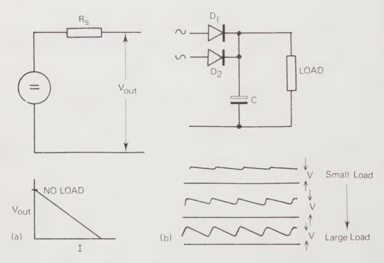
Fig. 5.9 THE CAUSES OF POOR REGULATION.
