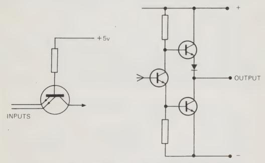
Fig. 9.4 The TTL (TRANSISTOR-TRANSISTOR-LOGIC) IC.
