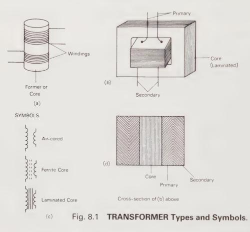
*Example.* A transformer has 7500 turns in its primary winding and is connected to a 250V 50 Hz supply. What a.c. voltage will be developed across its secondary winding if the latter has 500 turns?
