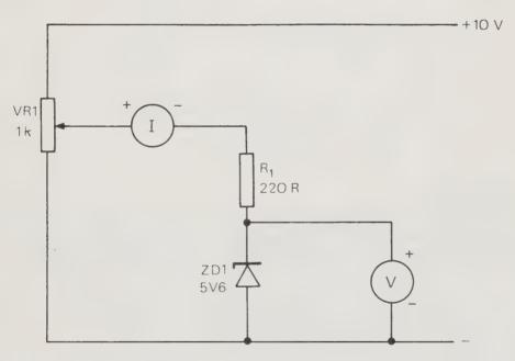
Fig. 2.5 ZENER DIODE Measurements.
