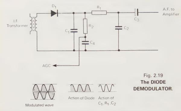
The high radio frequency is shorted to ground by  $C_1$ , and the low-pass filter  $R_1$ - $C_2$  removes any remaining trace of radio frequency from the output signal. Capacitor  $C_3$  is used to couple the signal to the next stage of amplification.
