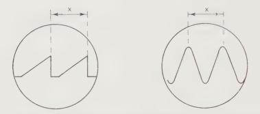
Fig. 1.8 Measuring the DURATION of a cycle of A.C.
