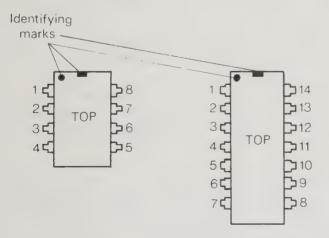
Fig. 3.20 **PIN-NUMBERING** Systems for Integrated Circuits.
