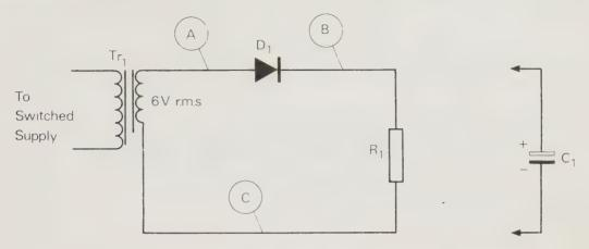
Fig. 2.9 A Measuring Circuit for the Half-wave Rectifier.
