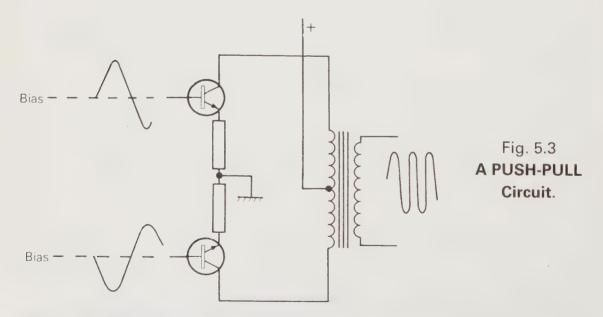
Both transistors feed current through the transformer, but in opposite directions. The transformer then combines the two outputs.
