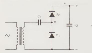
Fig. 5.15 A VOLTAGE-DOUBLER Circuit.
