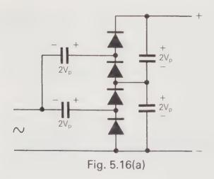
Fig. 5.16 The VOLTAGE-QUADRUPLER (a) Circuit: Alternative Configurations (b).
