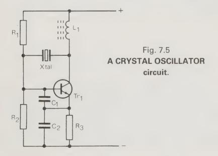
In normal use, crystal oscillators are extremely reliable, but excessive signal current flowing through the crystal can cause it to break down and fail. The usual comments concerning bias and decoupling components apply here also.
