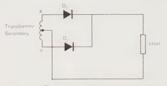
Fig. 2.10 FULL-WAVE RECTIFIER Circuit with Centre-tapped Transformer.
