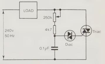
Fig. 3.17 The DIAC. Symbol and Typical Connection.
