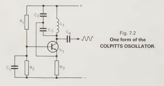
the combination of  $C_2$  and  $C_3$  to tap off a fraction of the output voltage to feed back into the base. This latter is biased and by-passed in the same way as in the Hartley circuit.
