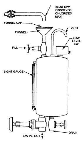
Figure 1-11.-Gravity expansion tank.
