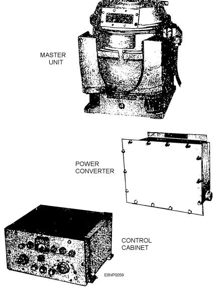
Figure 4-3.—Mk 27 Mod 0 gyrocompass equipment.
