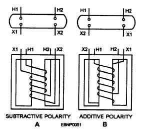
F'igure 3-17.-Polarity markings for large tramsformers: A. Subtractive polarity; B. Additive polarity.
