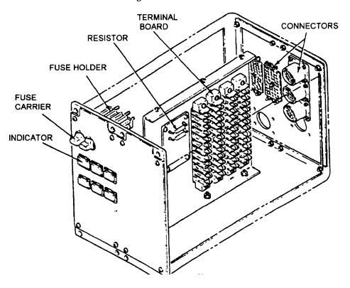
Figure 5-7.—Power distribution panel assembly.
