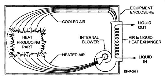
Figure 1-5.—Air-to-liquid cooling.
