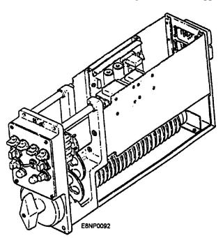
Figure 5-26-Remotely operated JR switch panel assembly.
