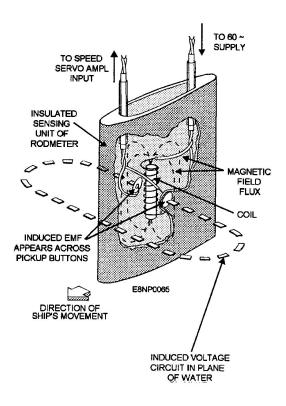
Figure 4-9.-Rodmeter sensing unit.
