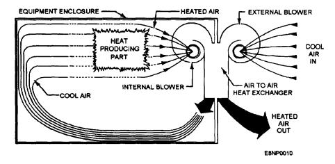
Figure 1-4.—Air-to-air cooling.
