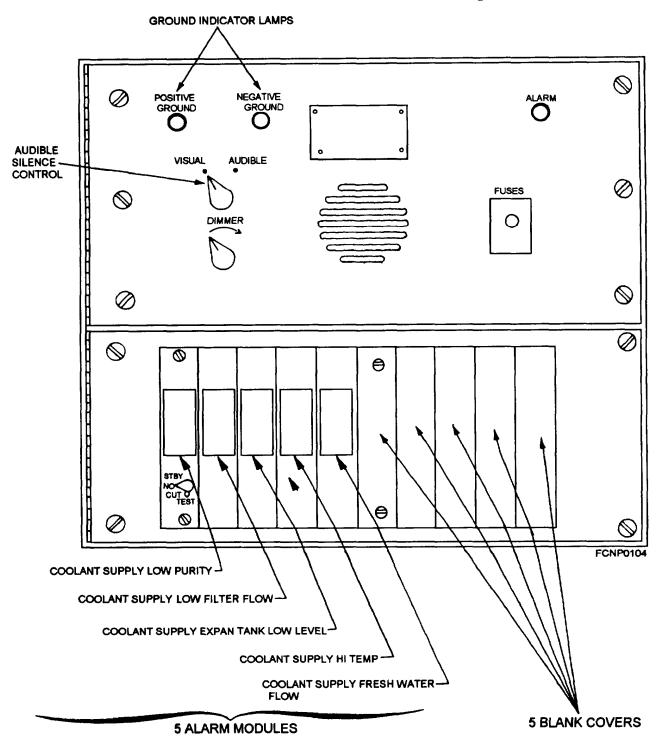
Figure 1-27.-Cooling system alarm switchboard.
