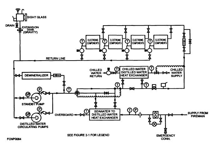
Figure 1-7.—Type II liquid cooling system.
