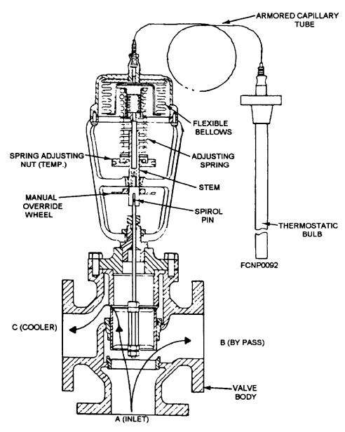
Figure 1-15.—Three-way temperature regulating valve.
