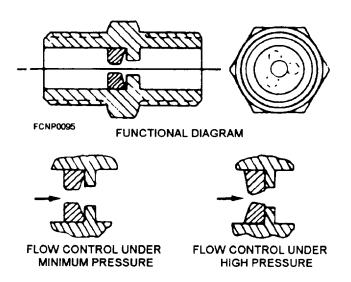
Figure 1-18.—Equipment flow regulator.
