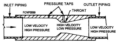
Figure 1-22.-Venturi flowmeter.
