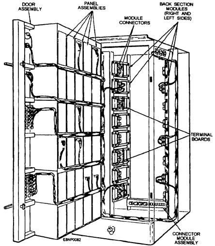
Figure 5-16.—Analog switchboard section, door open.
