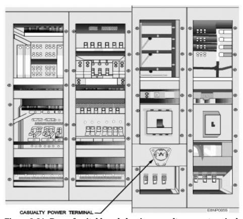
Figure 3-21.-Rear of switchboard showing casualty power terminal.
