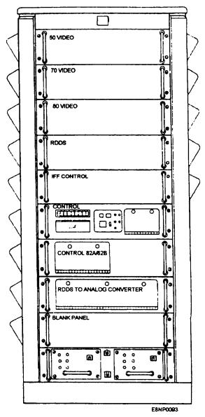
Figure 5-27.—Radar Distribution Switchboard, SB-4229/SP.
