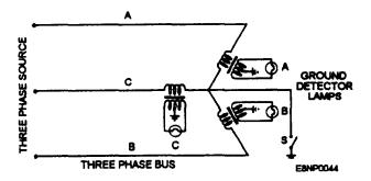
Figure 3-10.-An ac ground detector lamp circuit.
