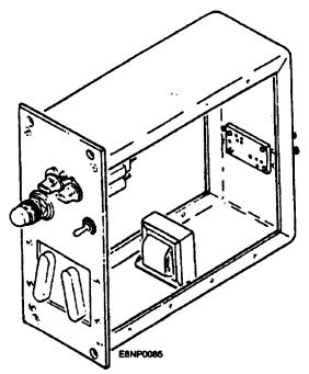
Figure 5-19.-Fuse tester assembly (analog switchboard).
