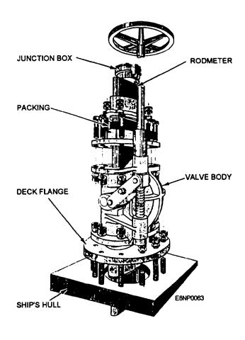
Figure 4-7.—Exploded view of theses valve.
