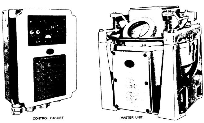
Figure 4-2.—Mk 23 Mod 0 gyrocompass equipment.
