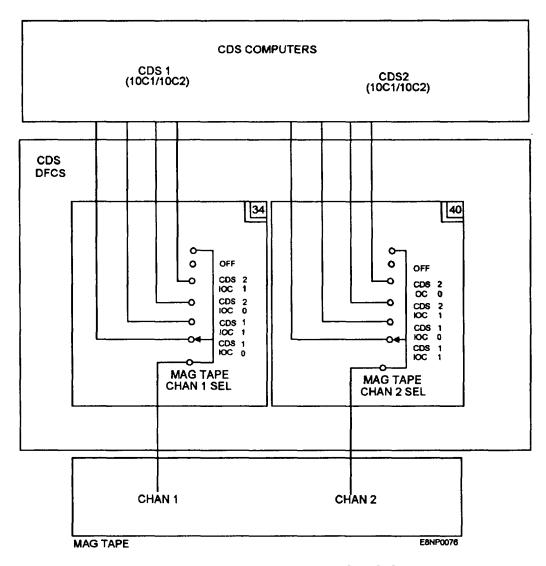
Figure 5-10.—Magnetic tape Interconnection through the DFCS.
