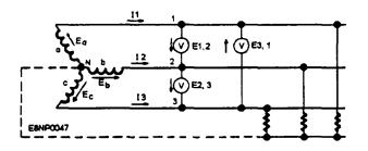
Figure 313.—Three-phase ac generatar showing neutral connection.
