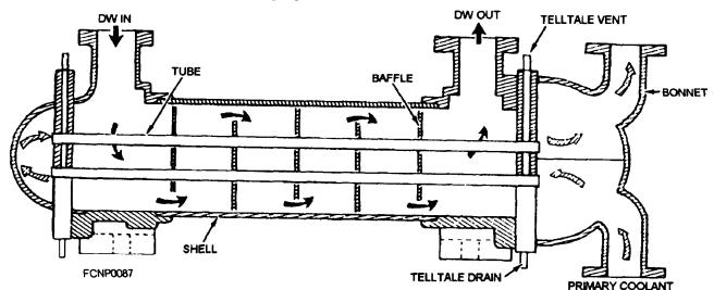
Figure 1-10.—Two-pass SW/DW beat exchanger with single-tube sheets.
