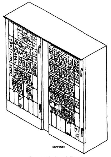
Figure 5-15.-Analog switchboard.
