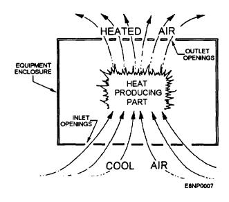
Figure 1-1.-Convection cooling.
