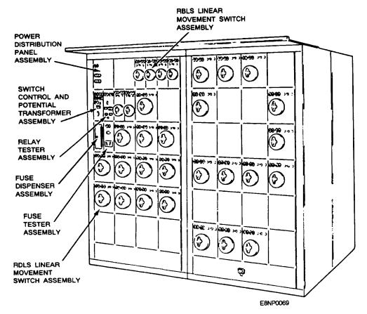
Figure 5-3.—Digital fire control switchboard (DFCS).
