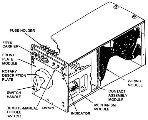
Figure 5-8.-R3DLSO-1B/R5DLSO-1B linear movement switch assembly.
