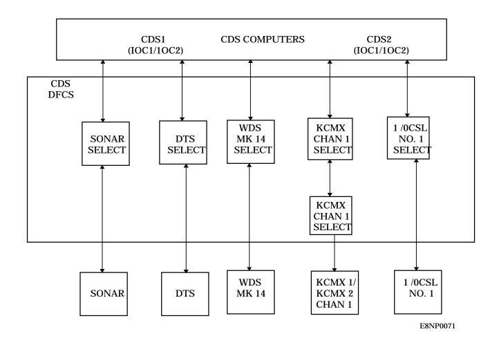
Figure 5-5.—Equipment interconnection through the CDS DFCS.
