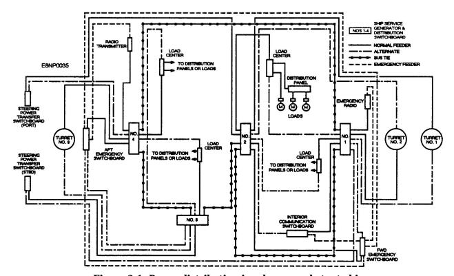
Figure 3-1.-Power distribution in a large combatant ship.
