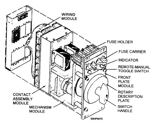
Figure 5-9.—R3BLSO-1C/R5BLSO-1C linear movement switch assembly.
