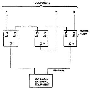
Figure 5-2.-Sample manual switching configuration.
