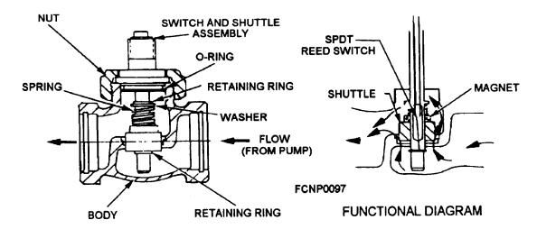
Figure 1-20.-Cooling system flow switch.
