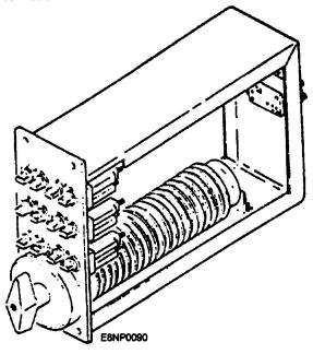
Figure 5-24.-Manually operated JR switch panel assembly.
