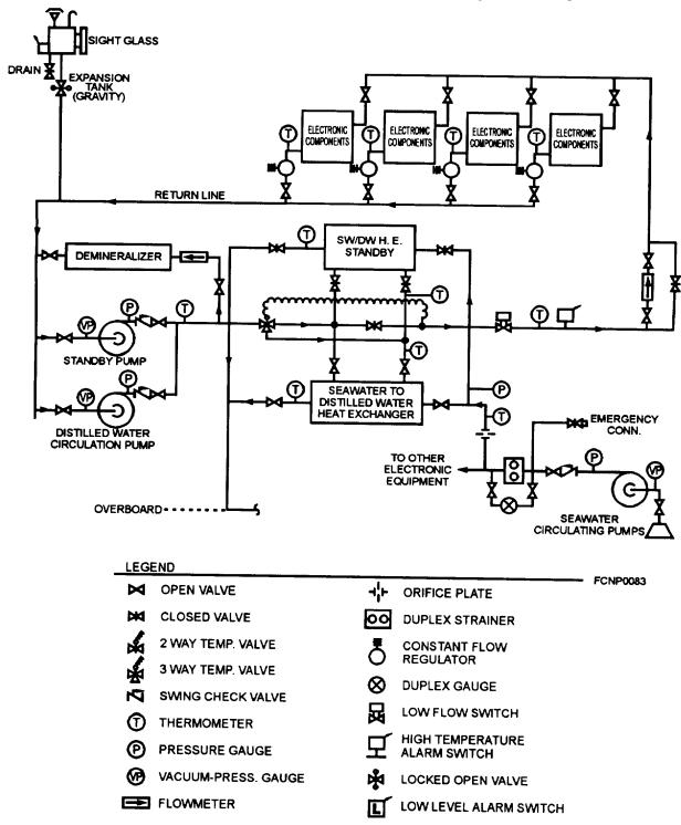
Figure 1-6.—Type I liquid cooling system.
