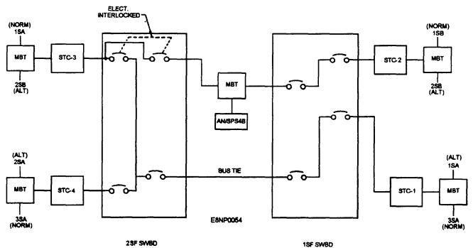
Figure 3-20.-400-Hz electric power distribution system.
