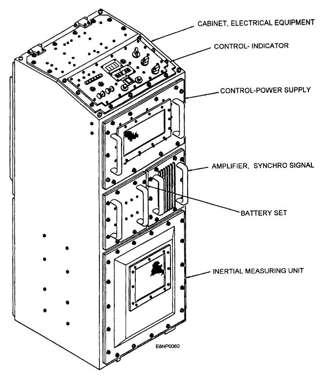
Figure 4-4.-Stabilized Gyrocompass Set AN/WSN-2.
