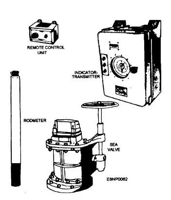
Figure 4-6.—Major components of the underwater log system.
