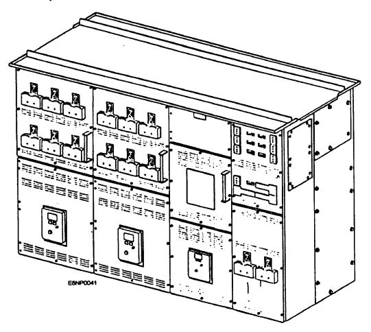
Figure 3-7.-1SB ship's service switchboard.
