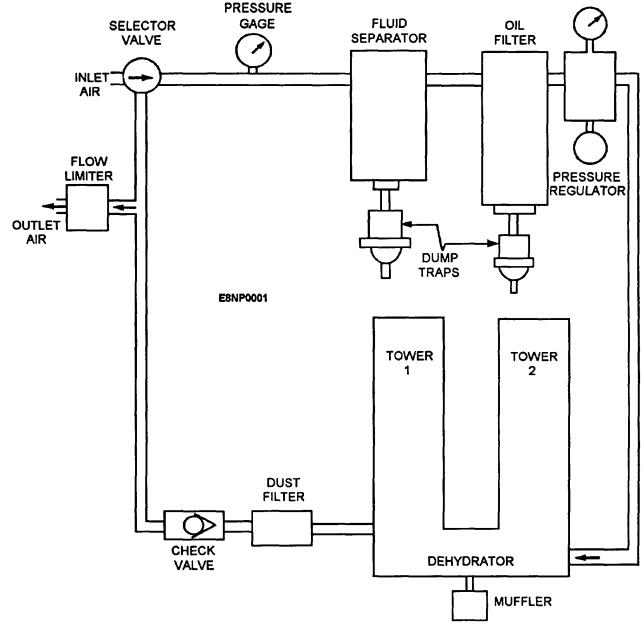
Figure 2-1.-Desiccant air dryer.
