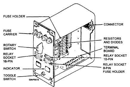
Figure 5-12.—Relay tester assembly,
