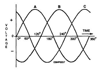
Figure 3-3.-Sine curve for three-phase circuit.
