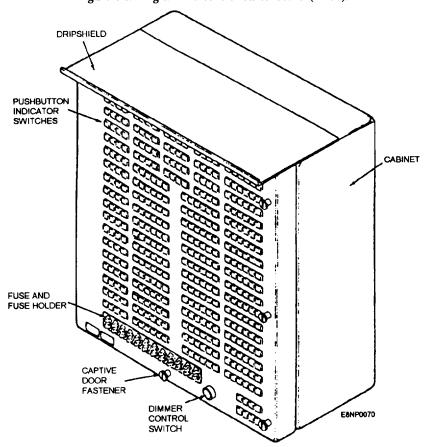
Figure 5-4.-Computer switching and control panel (CSCP).
