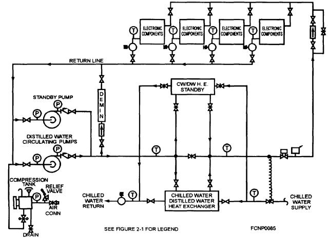
Figure 1-8.—Type III liquid cooling system.
