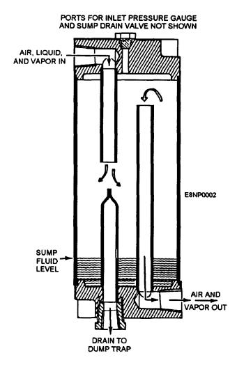
Figure 2-2.—Fluid separator.
