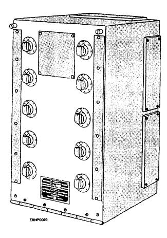
Figure 5-29.—Transmitter Transfer Switchboard. SB-988/SRT.
