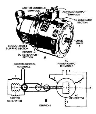
Figure 3-11.-An ac generator and schematic.
