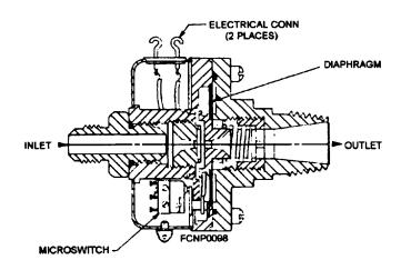
Figure 1-21.—Equipment flow switch.
