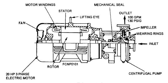
Figure 1-24.—Distllled water circulating pump.
