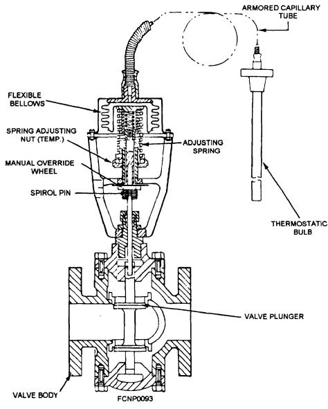
Figure 1-16.—Two-way temperature regulating valve.
