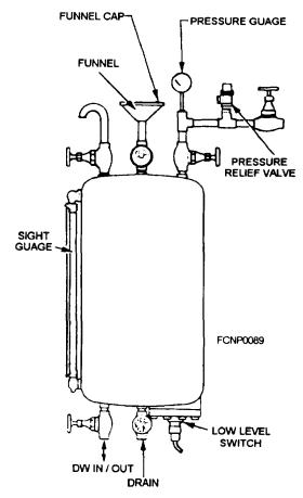
Figure 1-12.—Pre-ssure expansion tank.
