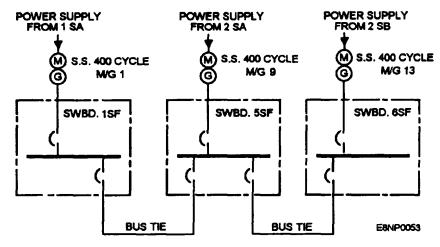
Figure 3-19.-Bus the connections on 400-Hz ship's service system.
