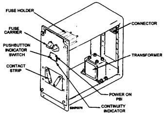
Figure 5-13.-Fuse tester assembly (DFCS).
