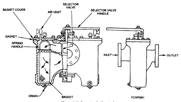
Figure 1-14.-Seawater duplex strainer.
