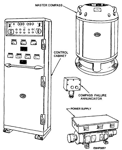
Figure 4-1.—Mk 19 Mod 3A gyrocompass equipment.
