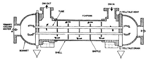
Figure 1-9.-Single-pass SW/DW heat exchanger with double-tube sheets.
