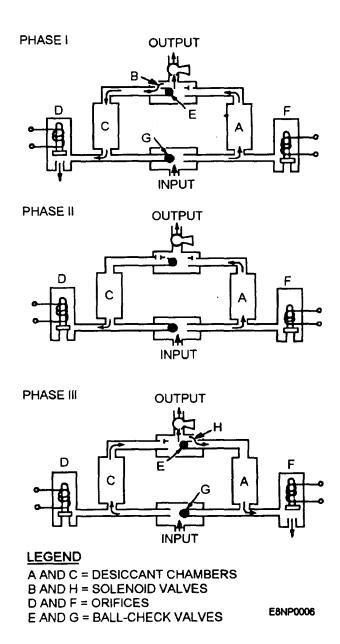
Figure 2-6.—Dehydrator operating cycle.
