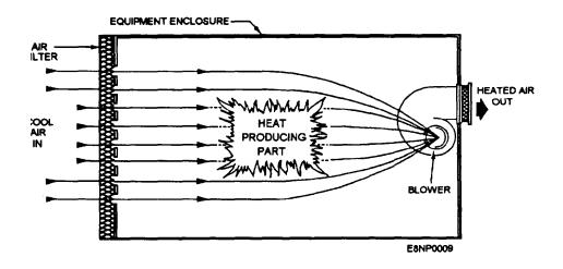
Figure 1-3.—Forced-air coding.
