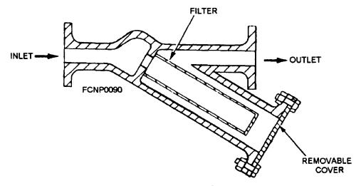
Figure 1-13.-Seawater simplex strainer.
