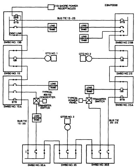
Figure 3-2.-Power distribution in a gas-turbine powered DDG.
