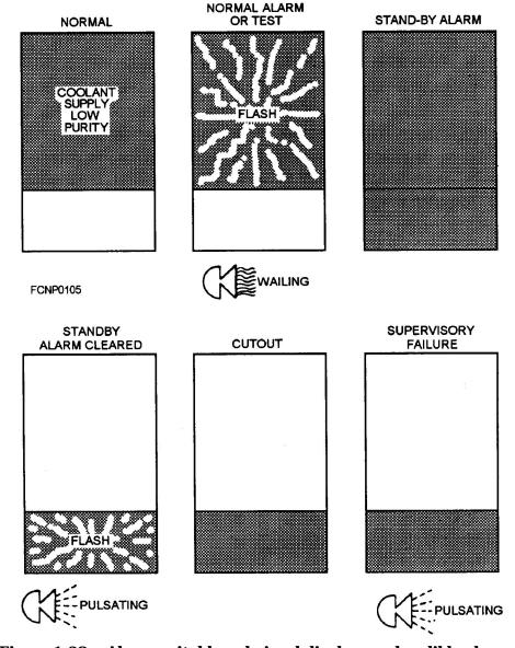
Figure 1-28.—Alarm switchboard visual displays and audible alarms.
