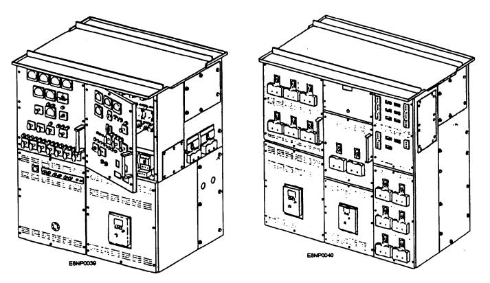
Figure 3-5.-1S ship's service switchboard.
