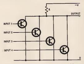
Fig. 11.4a. Bosic circuit of a transistor NOR gate
