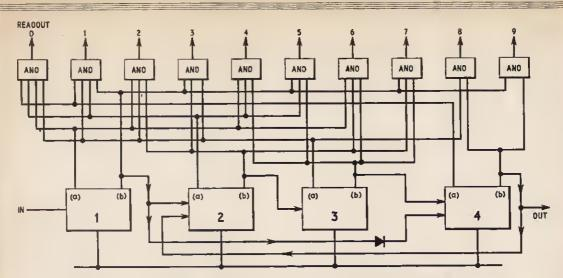
Fig. 11.3b. Cambination of the four binary bistable circuits and the AND gate decoder
