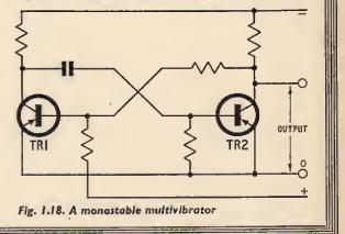
applied, as in the case of the bistable multivibrator, but after a predetermined time the circuit will again revert to its first state, as in the case of the astable multivibrator.
