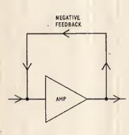
Fig. 1.10. A "block" diagram of amplifier with negative feedback
