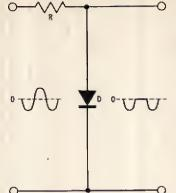
Fig. 1.8b. Diode limiter or clipper, positive part of signal clipped
