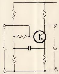
Fig. 1.14a. Basic "bootstrap" impedance amplifier
