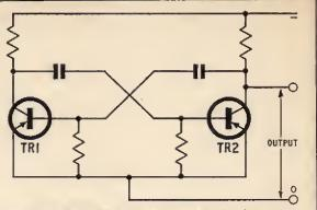
Fig. 1.16. An astable or free running multivibrator
