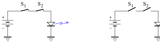
Figure 2.2. Electric circuit corresponding to the AND gate
