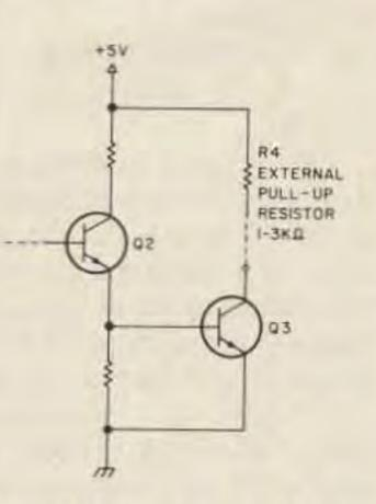
Fig. 4(b). An open-collector TTL circuit results when the output circuit is simplified. An external resistor is needed between the output and +5 volts.
