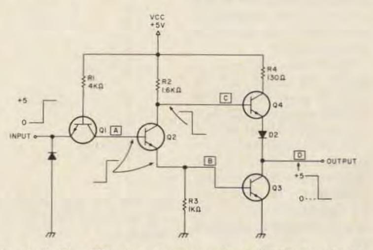
Fig. 4(a). The TTL (transistor-transistor logic) family has LOW values ranging from 0 to 0.8 volts. HIGH is 2.4 to 5.0
