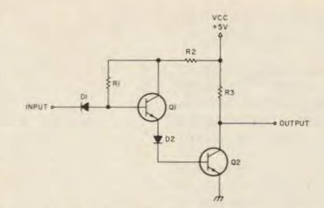
Fig. 3. DTL (diode-transistor logic) offers better speed than RTL. A typical DTL inverter is shown here.
