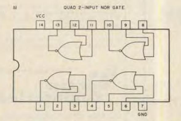
Fig. 9. A chip may contain as many as six individual gates. 78 73 Magazine • September, 1982 4) If A and B are both HIGH, then the output is LOW.
