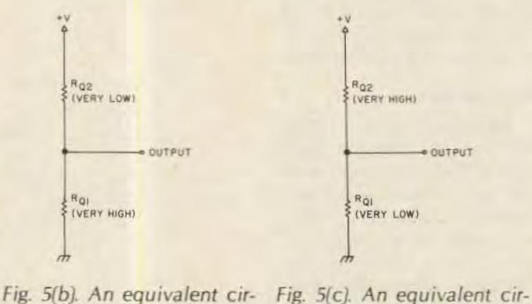
cuit for LOW input, HIGH cuit for HIGH input, LOW output. output.
