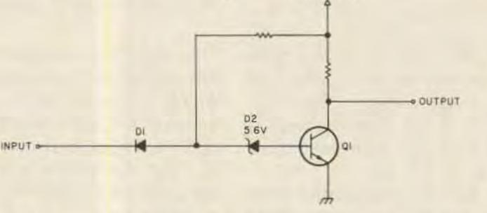
Fig. 6. HTL (high-threshold logic) is useful in applications where noise pulses may be a problem.
