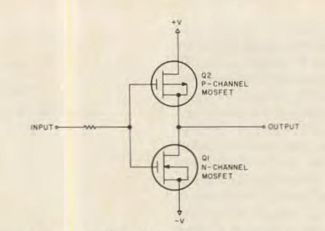
Fig. 5(a). A typical CMOS inverter circuit.
