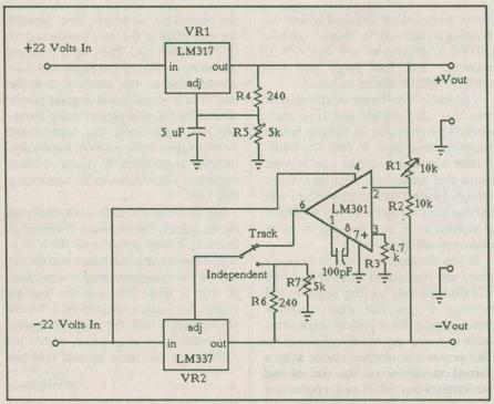
Figure 4. The Dual Tracking Regulator
