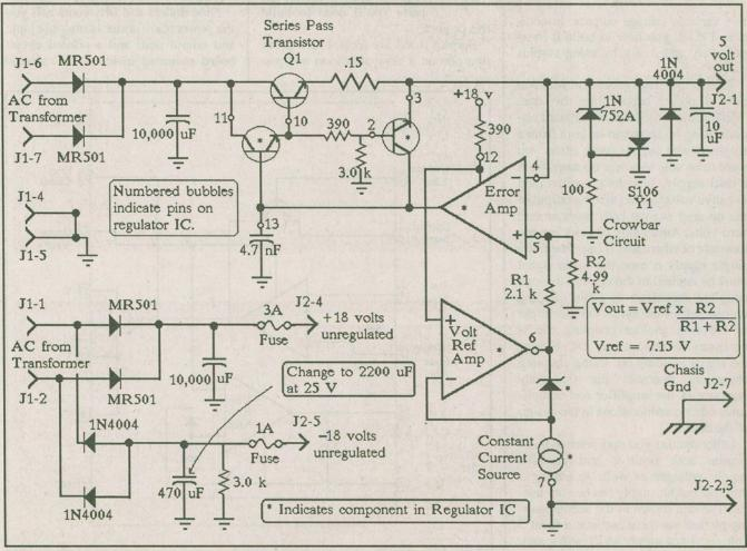
Figure 1. Schematic of Surplus Power Supply
