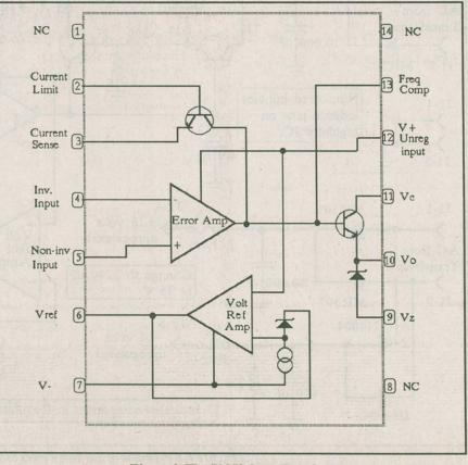
Figure 3. The 723 Voltage Regulator
