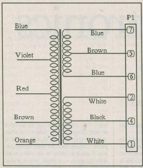
Figure 2. The Step Down Transformer
