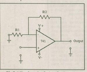
Fig. 3. A Non-Inverting Op Amp Configuration
