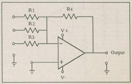
Fig. 7. A Summing Amplifier Configuration
