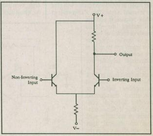
Fig. 2B. The Differential Amp Input Circuit
