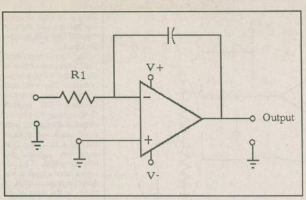
Fig. 8. An Integrator Configuration
