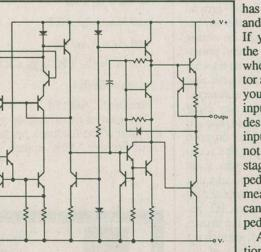
Fig. 2A. Internal Schematic of a 741 Op Amp
