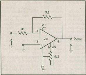
Fig. 3. An Inverting Op Amp Configuration
