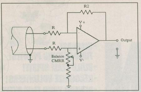
Fig. 4B. A Balanced Differential Amplifier
