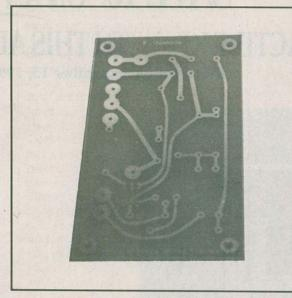
Figure 6. The Finished Printed Circuit Board
