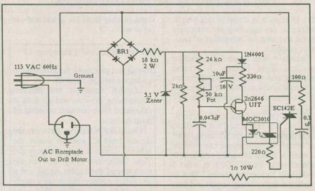
Figure 1. Variable Motor Speed Control Schematic with Corrections
