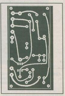
Figure 4. Negative of Printed Circuit
