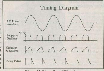
Figure 12. Phase Contol Waveforms
