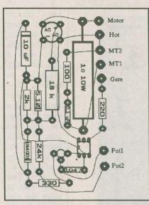
Figure 2. Component Side of PC
