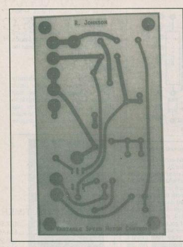
some places) created using this method. Using a light table with a grid on top, (tenths of an inch, yet even not metric!), and a sheet of mylar, the pads and tape are positioned on the mylar in the configuration required. This is all done at twice the size the board will eventually be (sometimes at four times the size for complex boards). When the artwork is finished, it is taken to a specialty photographic shop
