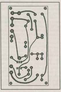
Figure 3. Solder Side of PC Board
