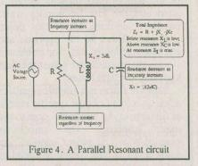
is the parallel circuit. Figure 4 shows a parallel resonant circuit in which the resistance, inductance and capacitance are connected in parallel with, in this case, a variable frequency current source. In this circuit the individual components behave in exactly the same way as before, but because they are in parallel we obtain a different result.
