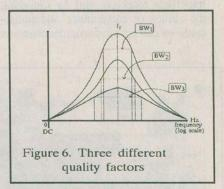
tive the circuit is. Figure 6 shows three different resonant responses superimposed on each other, all centred on the same frequency but with different quality factors. In order to determine the bandwidth (range of frequencies passed) of the circuit we use what are called the half-power points on the response curve. Half-power points are the point on the curve where the amplitude of the frequency at that point
