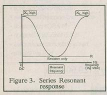
the circuit. See Figure 3. Naturally the opposition to current flow at this point is at a minimum and so current is max-
