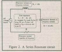
We said in the last segment that voltage leads current in the inductor and vice versa in the capacitor and the resistor just limits the current the same at all frequencies. We also said that ultimately the level of current and its phase shift with respect to the input voltage was determined by a combination of all the components and could only really be determined using vector algebra.
