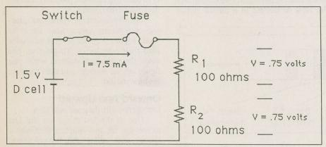
Fig. 6. A series circuit with two resistances.
