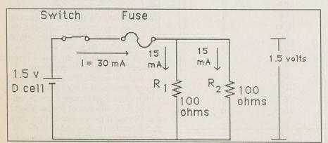
Fig. 7. A parallel circuit.
