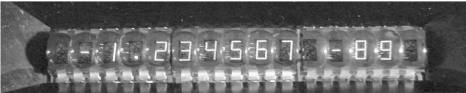
Fig. 12.3 An early LED calculator display with its very small digits which show red. The lenses over each one can just be seen. Source: https://en.wikipedia.org/wiki/Calculator#/media/File:LED_DISP.JPG
