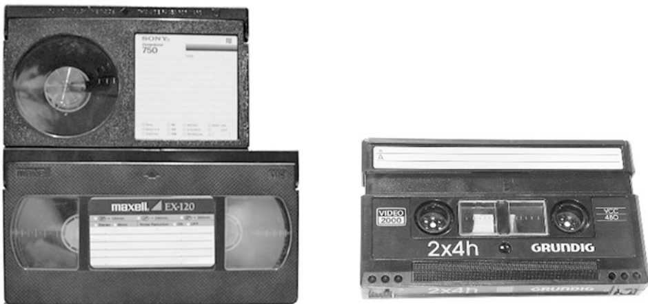
Fig. 25.1 Betamax cassette ( top ) and VHS ( below ) and a Philips Video 2000 cassette ( right ). Source: https://en.wikipedia.org/wiki/VHS#/media/File:Betavhs2.jpg ; https://en.wikipedia.org/wiki/Video_2000#/media/File:Grundig-Video2000-VCC-Kassette-1983-Rotated.jpg
