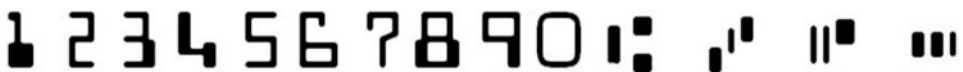
Fig. 24.1 The 14 magnetic ink characters used on cheques so that they could be read by machine. Source: https://en.wikipedia.org/wiki/Magnetic_ink_character_recognition#/media/File:MICR_char.svg
