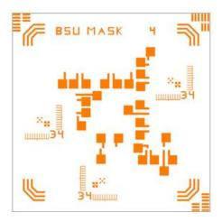
Figure 90. BEOL mask 4, top electrode definition
