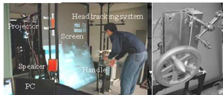
Figure 1. VR system for transmission of lathe operating skill
