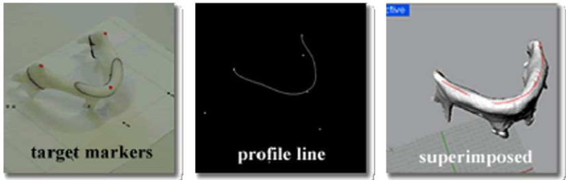
Figure 6. Regeneration of profile line and its superimposed image on the original data
