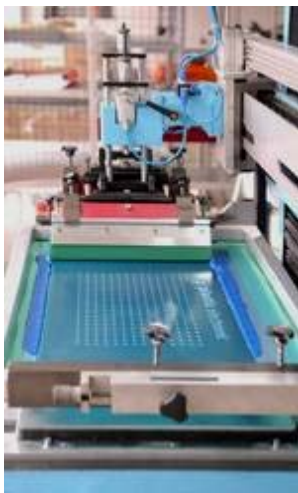
Figure 6.2. Screen printing equipment for large feature devices (courtesy of Plastic Electronic GmbH).
