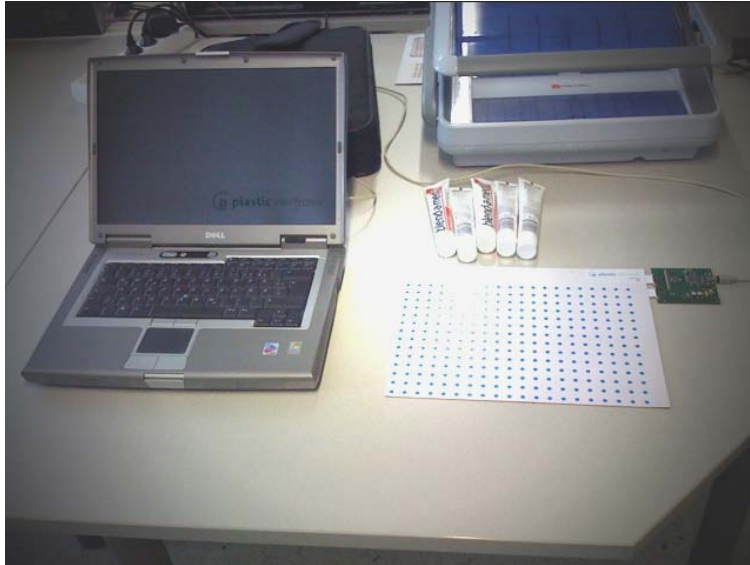
Figure B.6. Smart Shelf product prototype of Plastic Electronic company: A capacitive embedded film to sense the presence and location of products.
