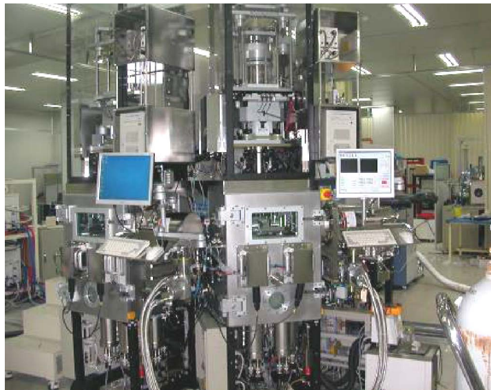
Figure 6.8. Pilot-scale vacuum-processing manufacturing platform (courtesy of Fraunhofer IPMS).
