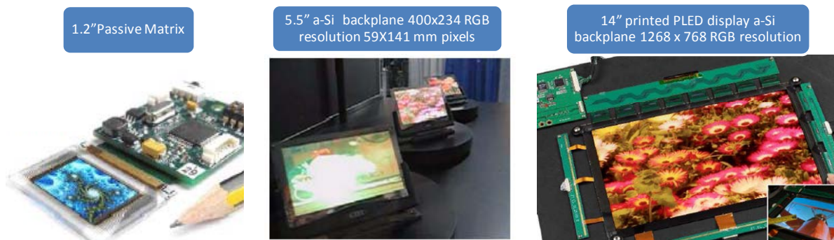
Figure 5.2. Display prototypes printed at CDT to demonstrate PLED manufacturing capabilities.
