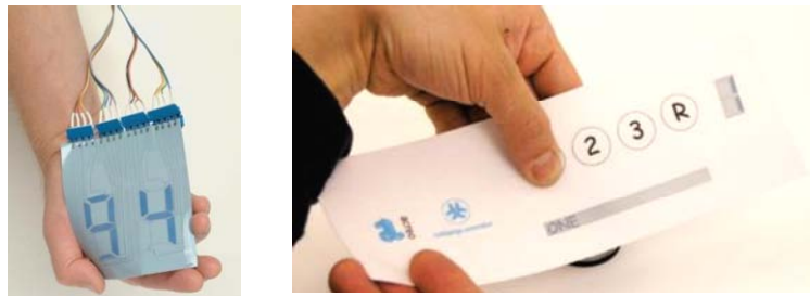
Figure 5.13. Electrochromic displays printed on paper and an integrated system with pressure switches, printed battery, and printed display.
