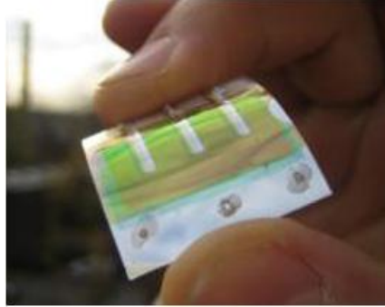
Figure 5.5. Flexible organic solar cell on metal foil (courtesy of Heliatek).
