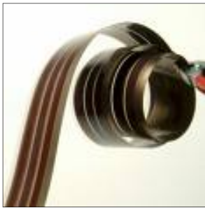
Figure 5.6. Konarka flexible organic photovoltaic cells manufactured via a roll-to-roll process (courtesy of Konarka).
