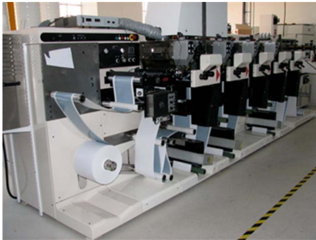
Figure 6.4. Roll-to-roll process prototyping platform developed from a commercial label printer (courtesy of ACREO).
