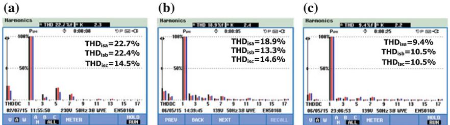
**Fig. 5.11** Experimental source current spectra **a** before compensation, **b** after the state-of-the-art control method compensation [18] and **c** after the proposed control method compensation
