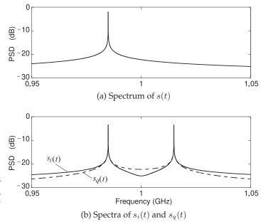
**Figure 3-30:** Spectra of the modulated signal with  $f_{\rm LO} = 1$  GHz. (Simulated time = 65.536 µs,  $2^{23}$  point FFT.)
