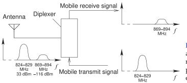
**Figure 5-3:** A diplexer which separates receive and transmit signals. A diplexer is a type of duplexer. However not all duplexers are diplexers.
