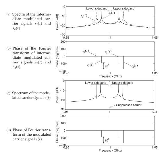
**Figure 3-28:** Spectrum of signals in the quadrature modulator of Figure 3-23(a) with 10 MHz inphase, i(t), and 15 MHz quadrature-phase, q(t), modulating signals. (Simulated time = 65.536 µs, using a 2<sup>23</sup> point FFT.)
