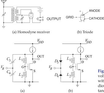
**Figure 3-4:** Colebrook's original homodyne receiver: (a) circuit with an antenna, tunable bandpass filter, and triode amplifier; and (b) triode vacuum tube.
