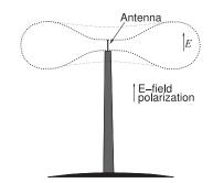
**Figure 4-10:** Field pattern produced by a microstrip antenna.
