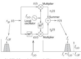
(b) SSB-SC modulator with IF input signal  $s_{\rm IF}(t)$
