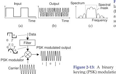
Figure 2-12: Binary PSK modulation: (a) modulating bitstream; (b) the modulated waveform; and (c) its spectrum after smoothing the transitions from one phase state to another.
