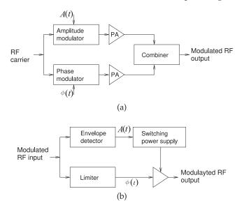
**Figure 3-14:** Polar modulator architectures: (a) amplitude- and phase-modulated components amplified separately and combined; and (b) the amplitude used to modulate a power supply driving a saturating amplifier with phase modulated input.
