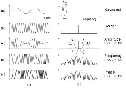
Figure 2-3: Basic analog modulashowing tion the waveform (i) and (ii) spectrum for (a) baseband signal; (b) carrier; (c) carrier modulated using amplitude modulation; carrier (d) modulated using frequency modulation; and (e) carrier modulated using phase modulation.
