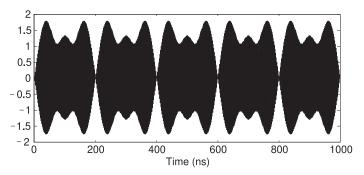
**Figure 3-27:** A 1 GHz carrier modulated by a 10 MHz sinusoidal i(t) and a 15 MHz sinusoidal q(t).
