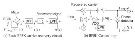
Figure 2-18: Block diagram of carrier recovery circuits for BPSK signals.
