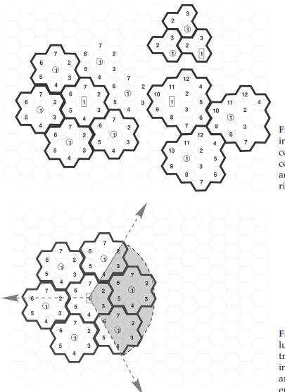
**Figure 4-24:** Cells arranged in clusters. Shown are 3cell clusters (top right), 7cell clusters (bottom left), and 12-cell clusters (bottom right).
