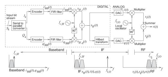
**Figure 3-40:** Complete SDR transmitter with bistream  $S_k$  input to an IF quadrature modulator producing a DSB-SC signal,  $s_{\rm IF}$ , with IF carrier of frequency  $f_{c,\rm IF}$ . Each finite-impulse response (FIR) filter implements raised cosine filtering. Then an analog SSB-SC quadrature modulator upconverts the IF as a DSB-SC RF signal centered at the RF carrier frequency  $f_c = f_{\rm LO} - f_{c,\rm IF}$ . The Hilbert transform implements a 90° phase shift.
