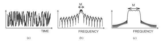
**Figure 2-26:** Details of digital modulation obtained using differential phase shift keying ( $\pi/4$ -DQPSK): (a) modulating waveform; (b) spectrum of the modulated carrier, with M denoting the main channel; and (c) details of the spectrum of the modulated carrier focusing on the main channel.
