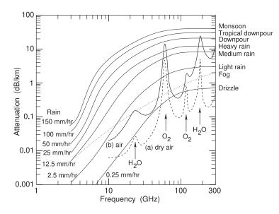
**Figure 4-18:** Excess attenuation due to atmospheric conditions showing the effect of rain on RF transmission at sea level. Curve (a) is atmospheric attenuation, due to excitation of molecular resonances, of very dry air at 0 °C, curve (b) is for typical air (i.e. less dry) at 20 °C. The attenuation shown for fog and rain is additional (in dB) to the atmospheric absorbtion shown as curve (b).
