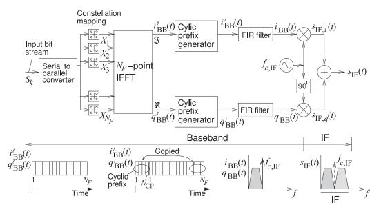
Figure 5-22: Block diagram of an OFDM modulator.
