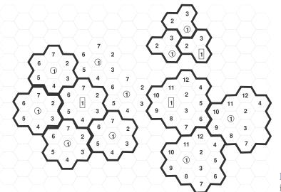
**Figure 5-4:** Cells arranged in clusters.
