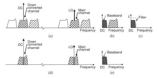
**Figure 3-16:** Frequency conversion using homodyne mixing: (a) the spectrum with a large LO and the low frequency products after down conversion; (b) the baseband spectrum showing only positive frequencies; (c) the baseband spectrum after mixing; (d) down conversion spectra when the radio signal has no spectral content at the carrier frequency; and (e) the lowpass filtered down-converted signal in (d).
