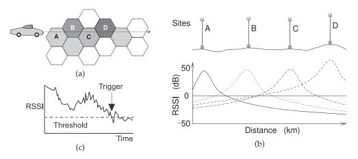
**Figure 5-7:** Process of handoff: (a) movement of a mobile unit through cells; (b) received signal strength indicator (RSSI) during movement of a mobile unit through cells; and (c) RSSI of a mobile unit showing the handoff triggering event.
