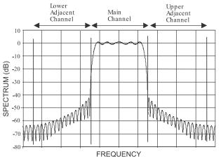
**Figure 2-27:** Detailed spectrum of a  $\pi/4$ -DQPSK signal showing the main channel and lower and upper adjacent channels.
