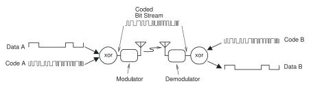
**Figure 5-14:** Depiction of direct sequence CDMA transmission. If code B is code A, then data B is the same as data A with some corruption by noise.
