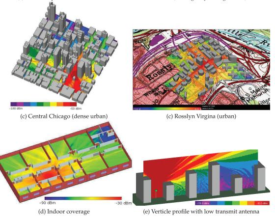
**Figure 4-28:** Radio coverage profiles with 900 MHz transmitter except for (d) which is for 2.45 GHz. Calculated using Wireless Insite<sup>®</sup>. Copyright Remcom, Inc. Used with permission.
