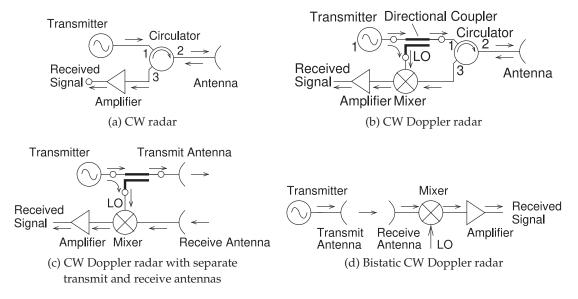
Figure 5-27: Radar architectures.
