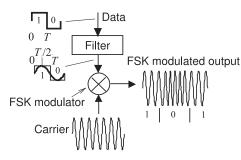
**Figure 2-10:** The frequency shift keying (FSK) modulation system. In the GSM four-state cellular systemadjacent constellation points differ in frequency by 33.25 kHz.
