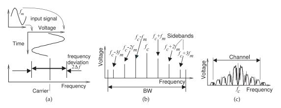
**Figure 2-7:** Frequency modulation: (a) sinusoidal baseband signal shown varying the frequency of the carrier and so FM modulating the carrier; (b) the spectrum of the resulting FM-modulated waveform; and (c) spectrum of the modulated carrier when it is modulated by a broadband baseband signal such as voice.
