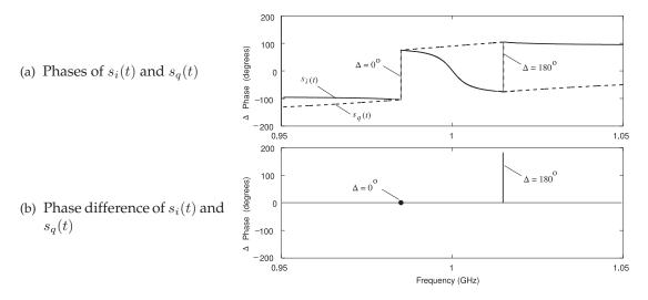
**Figure 3-31:** Phase of the modulated signal. (Simulated time =  $65.536 \,\mu$ s,  $2^{23}$  point FFT.)
