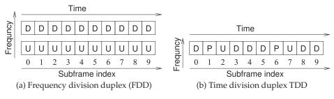
Figure 5-20: Duplex schemes used in 4G with ten subframes in a 10 ms frame.
