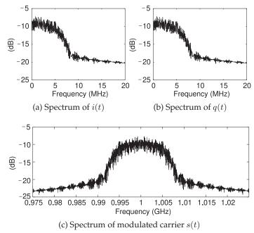
**Figure 3-36:** Spectra of signals in the digital modulator with a 20 Mbit/s input stream,  $S_k$ , and a 1 GHz LO. (1024 symbols, a time duration of 102.4 µs, and using a 524,288 point FFT)
