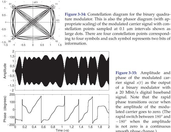
Figure 3-35: Amplitude and phase of the modulated carrier signal s(t) as the output of a binary modulator with a 20 Mbit/s digital baseband signal. Note that the rapid phase transitions occur when the amplitude of the modulated carrier goes to zero. (The rapid switch between 180° and  $-180^{\circ}$  when the amplitude is not zero is a continuous smooth phase change.)
