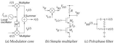
**Figure 3-23:** Quadrature modulator. The simple modulator in (b) is based on a FET cascode amplifier and the polyphase filter in (c) has a 90° phase difference between i(t) and q(t).
