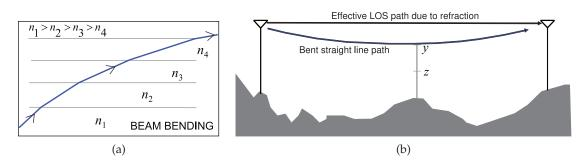
**Figure 4-21:** Beam bending by density variation in air: (a) refraction index profile with the air density reducing with height; and (b) incorporating beam bending in a curved-earth model.
