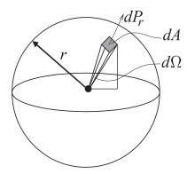
**Figure 4-9:** Free-space spreading loss. The incremental power,  $dP_r$ , intercepted by the shaded region of incremental area dA is proportional to  $1/r^2$ . The solid angle subtended by the shaded area is the incremental solid angle  $d\Omega$ . The integral of dA over the surface of the sphere, i.e. the area of the sphere is  $4\pi r^2$ . The total solid angle subtended by the sphere is the integral of  $d\Omega$  over the sphere and is  $4\pi$  steradians (or  $4\pi$  sr).
