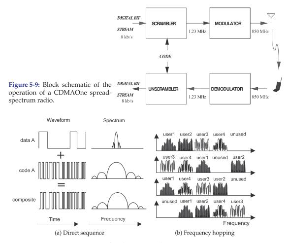
Figure 5-10: Basis of multiuser spread-spectrum communication.
