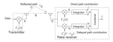
**Figure 5-16:** Rake receiver used to decode two paths, a direct path and a path with excess delay  $t_D$ . The integrators eliminate incorrectly recovered data.
