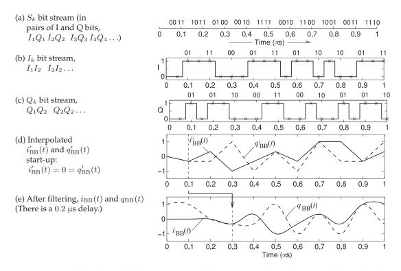
**Figure 3-42:** Baseband signals for 16-QAM modulation with markers showing the baseband bit impulse times. The bit pairs shown above each bit waveform 0.1 µs intervals.
