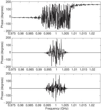
**Figure 3-38:** Phase of the FFT of the digitally modulated RF signal and its components. The phase of the  $s_i(t)$  and  $s_q(t)$  has been weighted by their spectrum amplitudes as otherwise meaningless numerical noise dominates the plots outside the passband. (Using 1024 symbols, 102.4 µs)
