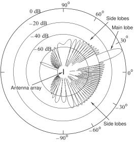
$_{0}$ ° **Figure 4-29:** Electric field pattern from a 30 element array of antennas spaced 0.65λ appart. The sidelobe levels are about 40 dB below the power level of the main lobe. The same signal is presented to the antenna elements except that phases of the signal at each antennas is adjusted to produce a main beam directed at 20 degrees. The signals to each antenna are thus correlated. After [29].
