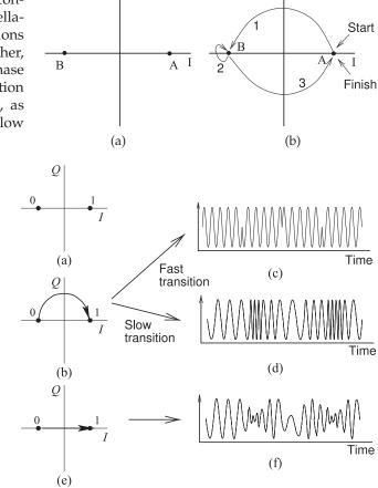
**Figure 2-17:** BPSK modulation: (a) constellation diagram; (b) constellation diagram with a constant amplitude transition; (c) time-domain waveform if the transition is fast; (d) time-domain waveform if the transition is slow; (e) constellation diagram with transition through the origin; and (f) time-domain waveform if the transition goes through the origin and is slow.
