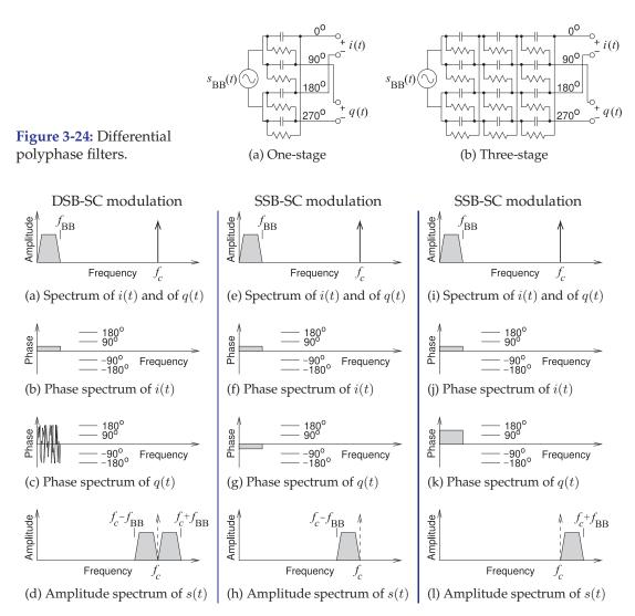
**Figure 3-25:** Spectra of the baseband i(t) and q(t) signals and the modulated s(t) signal, see Figure 3-23(a), for double sideband (DSB) and single sideband (SSB) suppressed-carrier (SC) modulation. Here the carrier frequency  $f_c = f_{LO}$ , the LO frequency in Figure 3-23(a).
