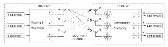
**Figure 5-21:** A MIMO system showing multiple paths between each transmit antenna and each receive antenna.
