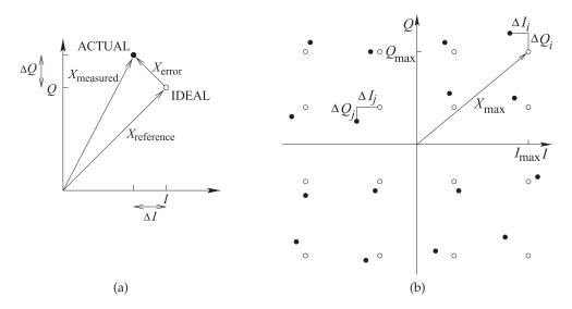
**Figure 2-37:** Partial constellation diagram showing quantities used in calculating EVM: (a) definition of error and reference signals; and (b) error quantities used when constellation points have different powers.
