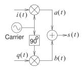
**Figure 2-15:** Quadrature modulator block diagram. In PSK modulation i(t) and q(t) have the same amplitude and indicate a phase  $\phi$  of the modulated carrier so that  $i(t) = \cos[\phi(t)]$  and  $q(t) = \sin[\phi(t)]$ . The particular example shows two possible values of  $I_k$  and  $Q_k$  and this indicates QPSK modulation.
