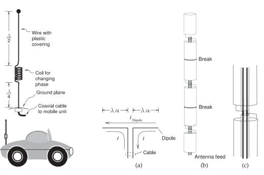
**Figure 4-6:** Mobile antenna with phasing coil extending the effective length of the antenna.
