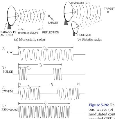
**Figure 5-25:** Radar system: (a) monostatic radar with the same site used for transmission of the radar signal and receipt of the reflection from the target; and (b) bistatic radar with different transmit and receive sites.
