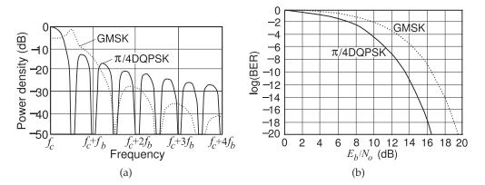
**Figure 2-36:** Comparison of GMSK and  $\pi/4$ DQPSK: (a) power spectral density as a function of frequency deviation from the carrier; and (b) BER versus signal-to-noise ratio (SNR) as  $E_b/N_o$  (or energy per bit divided by noise per bit).
