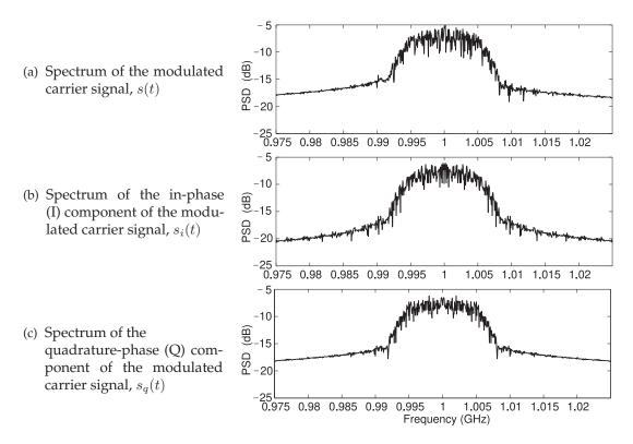
**Figure 3-37:** Spectra of the digitally modulated RF signals for 1024 symbols (4096 bits), a time duration of 102.4 µs, and using a 524,288 point FFT.
