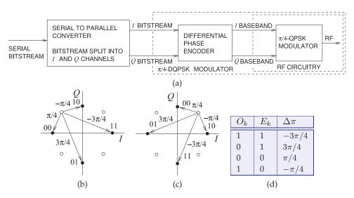
**Figure 2-24:** A  $\pi/4$ -DQPSK modulator: (a) differential phase encoder with a  $\pi/4$ -QPSK modulator; (b) constellation diagram of  $\pi/4$ -DQPSK; (c) a second constellation diagram; and (d) phase changes in a  $\pi/4$ -DQPSK modulation scheme. Note that the information is in the phase change rather than the phase state.
