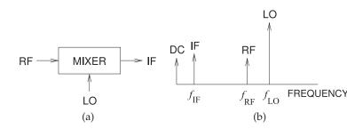
**Figure 3-8:** Simple mixer circuit: (a) block diagram; and (b) spectrum.
