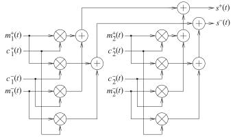
**Figure 3-10:** Differential implementation of a Hartley SSB-SC modulator:  $s^+(t)$ ,  $s^-(t)$  are the positive and negative components of the differential modulated signal s(t);  $(c_1^+(t), c_1^-(t))$  is the differential carrier;  $(m_1^+(t), m_1^-(t))$  is the differential quadrature-modulated IF carrier;  $(c_2^+(t), c_2^-(t))$  is the differential carrier shifted 90°; and  $m_2^+(t)$  and  $m_2^-(t)$  are the 90° phase-shifted versions of  $m_1^+(t)$  and  $m_1^-(t)$ , respectively.
