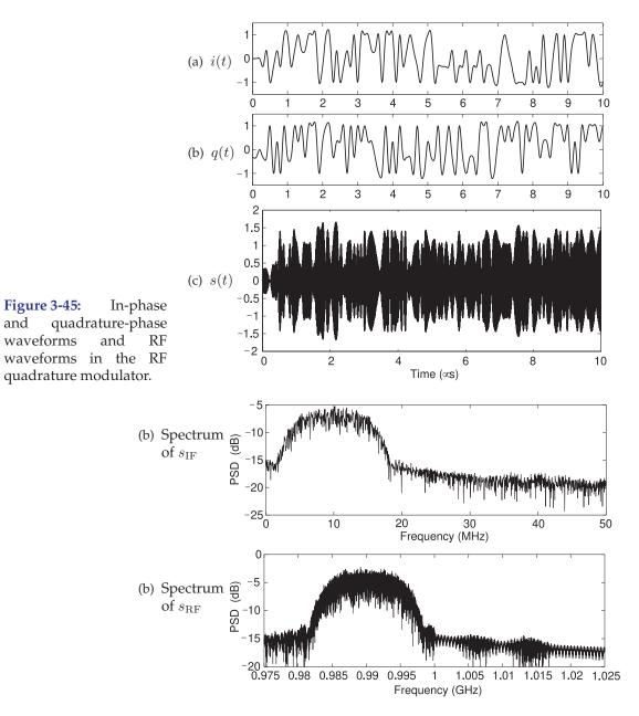
Figure 3-46: Spectrum of the IF and RF modulated carriers.
