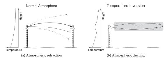
**Figure 4-19:** Fading resulting from ducting: (a) normal atmospheric refraction (normally the temperature of air drops with increasing height and the lower refractive index at high heights results in a concave refraction); and (b) atmospheric ducting (resulting from temperature inversion inducing an air layer with higher dielectric constant than the surrounding air).
