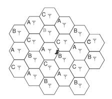
**Figure 4-26:** Base station with trisector stacked-dipole **Figure 4-27:** Three-cell cluster with motransmit and microstrip patch receive antennas. bile unit at the edge of cells A, B, and C.
