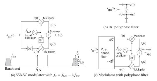
**Figure 3-29:** Quadrature modulator as a single-sideband, suppressed-carrier (SSB-SC) modulator. At the design frequency the polyphase filter in (b) the phase of i(t) is advanced by  $45^{\circ}$  and the phase of q(t) is retarded by  $45^{\circ}$ .
