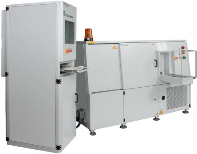
Fig. 2 Realised CT system for process integrated piston inspection within 30 seconds
