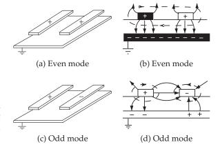
**Figure 6-2:** Modes on parallel-coupled microstrip lines. In (b) and (d) the electric fields are indicated as arrowed lines and the magnetic field lines are dashed.
