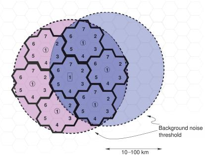
**Figure 1-9:** Interference in a cellular radio system.
