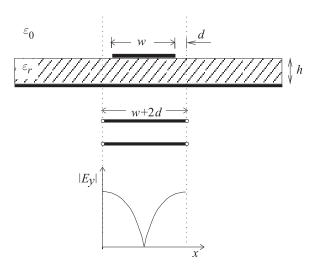
section of microstrip; and (b) microstrip Figure 5-11: Transverse resonance: standing wave waveguide model having effective width  $(|E_u|)$  and equivalent transmission line of length
