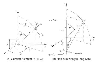
**Figure 2-3:** Wire antennas. The distance from the center of an antenna to the field point P is r.
