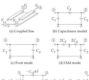
**Figure 6-5:** Very low frequency models of a pair of coupled lines.
