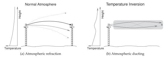
**Figure 2-15:** Fading resulting from ducting: (a) normal atmospheric refraction (normally the temperature of air drops with increasing height and the lower refractive index at high heights results in a concave refraction); and (b) atmospheric ducting (resulting from temperature inversion inducing an air layer with higher dielectric constant than the surrounding air).
