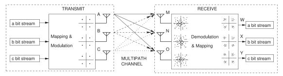
**Figure 2-18:** A MIMO system showing multiple paths between each transmit antenna and each receive antenna.
