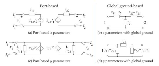
**Figure 7-2:** The *z*- and *y*-parameter equivalent circuits for port-based and global ground representations. The immittances are shown as impedances.
