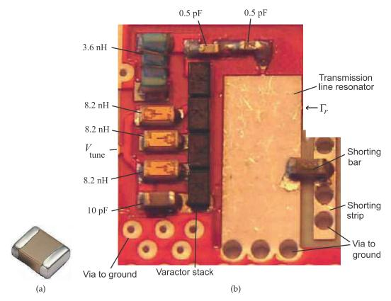
**Figure 9-4:** Circuit board showing the use of surface-mount components: (a) chip resistor or capacitor with metal terminals at the two ends; and (b) a populated RF microstrip circuit board of a 5 GHz tunable resonator [1]. The larger components have dimensions 1.6 mm  $\times$  0.8mm. The shorting bar is a 0  $\Omega$  chip resistor.
