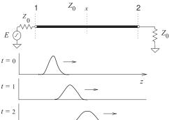
**Figure 5-2:** Dispersion of a pulse t = 2 along a line.
