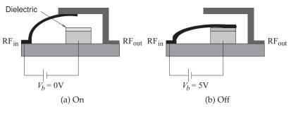
Figure 11-13: RF MEMS switch: (a) the  $RF_{\rm in}$  line in contact with the  $RF_{\rm out}$  line; and (b) the cantlever beam electrostatically attracted to the pedestal and there is no RF connection.
