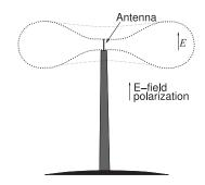
Figure 2-11: A base station transmitter pattern.
