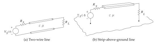
Figure 3-1: Two conductor transmission lines.
