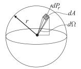
**Figure 2-9:** Free-space spreading loss. The incremental power,  $dP_r$ , intercepted by the shaded region of incremental area dA is proportional to  $1/r^2$ . The solid angle subtended by the shaded area is the incremental solid angle  $d\Omega$ . The integral of dA over the surface of the sphere, i.e. the area of the sphere is  $4\pi r^2$ . The total solid angle subtended by the sphere is the integral of  $d\Omega$  over the sphere and is  $4\pi$  steradians (or  $4\pi$  sr).
