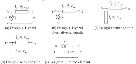
**Figure 10-45:** Matching network topologies using lumped elements and microstrip lines. In the stub layouts x is a via to the ground plane implementing a short circuit (s/c) and an open circuit o/c simply does not show a connection to the microstrip ground plane.
