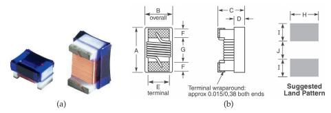
**Figure 9-5:** Chip inductor: (a) in an 0603 surface-mount package; and (b) schematic showing sizes and pads to be provided on a circuit board (A=64 mils (1.63 mm), B=33 mils (0.84 mm), C=24 mils (0.61 mm), D=13 mils (0.33 mm), E=30 mils (0.76 mm), F=25 mils (0.64 mm), G=25 mils (0.64 mm), and H=40 mils (1.02 mm)). Copyright Coilcraft, Inc., used with permission [2].
