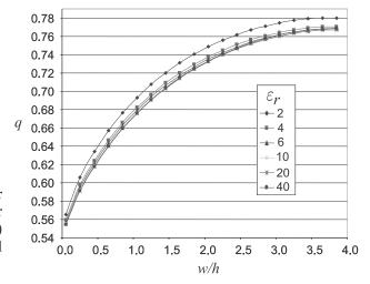
**Figure 4-7:** Dependence of the q factor of a microstrip line at 1 GHz for various permittivities and aspect (w/h) ratios. (Data obtained from EM field simulations using Sonnet.)
