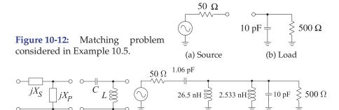
**Figure 10-13:** Matching network topology used in Example 10.5: a) and (b) topology; and (c) intermediate matching network.
