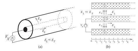
**Figure 3-2:** A coaxial transmission line: (a) three-dimensional view; (b) the line with pulsed voltage source showing the electric fields at an instant in time as a voltage pulse travels down the line.
