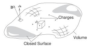
**Figure 1-6:** Diagram illustrating Gauss's law. Charges are distributed in the volume enclosed by the closed surface. An incremental area is described by the vector  $d\mathbf{S}$ , which is normal to the surface and whose magnitude is the area of the incremental area.
