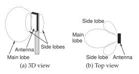
**Figure 2-10:** Field pattern produced by a microstrip antenna.
