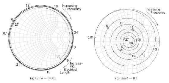
**Figure 8-18:** Smith chart plot of the reflection coefficient of the shorted 1 cm-long microstrip line in Figure 8-17: (a) a low-loss substrate with  $\tan \delta = 0.001$ ; and (b) a high-loss substrate with  $\tan \delta = 0.1$ . Frequencies are marked in gigahertz.
