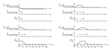
**Figure 3-3:** Fields, currents, and charges on the coaxial transmission line of Figure 3-2 at times  $t_4 > t_3 > t_2 > t_1$ .  $Q_{\rm CENTER}$  is the net free charge on the center conductor.  $I_{\rm CENTER}$  is the current on the center conductor.
