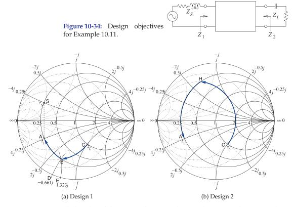
**Figure 10-35:** Smith chart-based designs used in Example 10.11. (50  $\Omega$  normalization used.)
