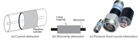
**Figure 9-9:** Distributed attenuators. The attenuators in (c) have power handling ratings of 2W, 5W and 20 W (left to right). Copyright 2012 Scientific Components Corporation d/b/a Mini-Circuits, used with permission [4].
