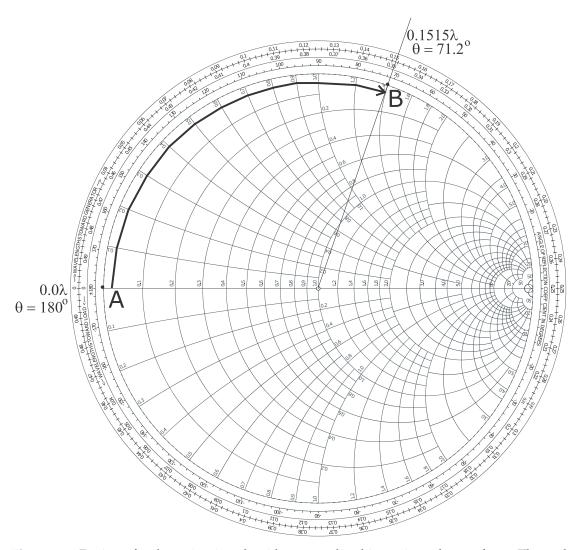
**Figure 8-7:** Design of a short-circuit stub with a normalized input impedance of  $\jmath 1.4$ . The path AB is actually on the unit circle but has been displaced here to avoid covering numbers. The electrical length in wavelengths has been read from the outermost circular scale, and the angle,  $\Theta$ , in degrees refers to the angle of the polar plot (and is twice the electrical length).
