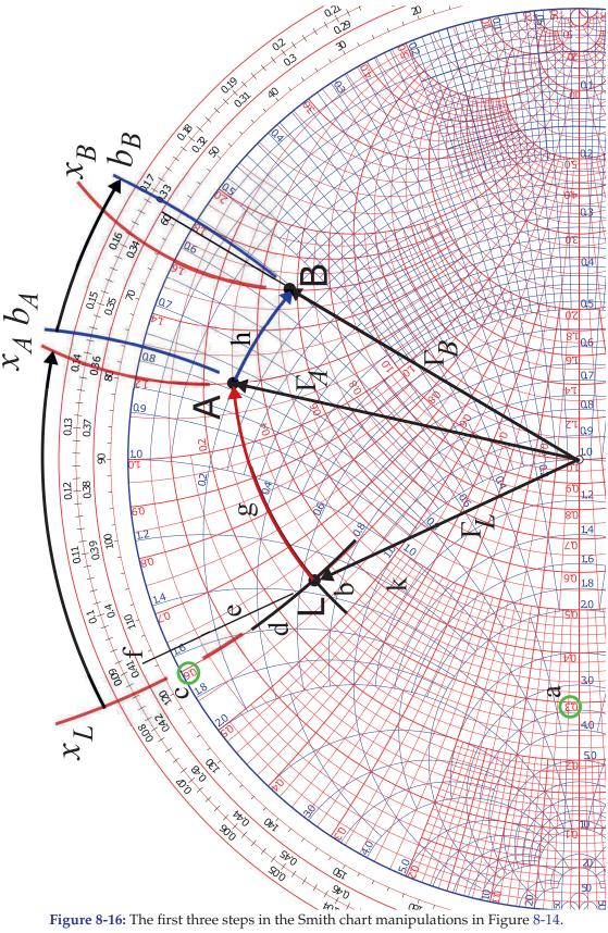
Smith chart so the susceptance must be negative even though a minus sign is not shown on the Smith chart. Thus the correct reading for  $x_A$  is -0.784. Now  $b_{BA} = +0.230$  so the locus, 'h', of the transition follows the circle of constant conductance ending at the (interpolated arc) with susceptance  $b_B = b_a + b_{BA} = -0.784 + 0.230 = -0.554$ .
