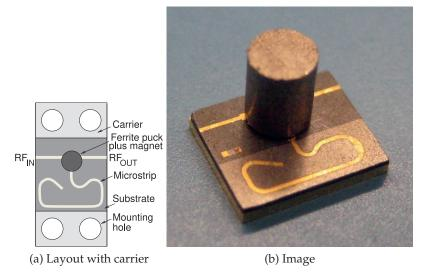
**Figure 11-17:** A microstrip isolator operating from 29 to 31.5 GHz. Isolator in (b) has the dimensions  $5 \text{ mm} \times 6 \text{ mm}$  and is 6 mm high. The isolator supports 2 W of forward and reverse power with an isolation of 18 dB and insertion loss of 1 dB. Renaissance 2W9 series, copyright Renaissance Electronics Corporation, used with permission.
