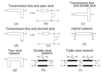
**Figure 10-37:** Matching networks with transmission line elements.
