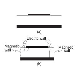
Figure 5-10: Approximation of a microstrip line as a waveguide: (a) cross w + 0.4h with magnetic and electric walls. w + 2d, where d = 0.2h.
