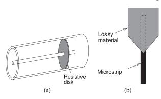
**Figure 9-6:** Terminations: (a) coaxial line resistive termination; (b) microstrip matched load.
