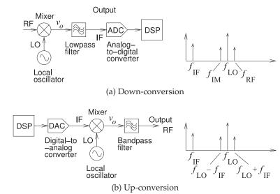
**Figure 11-18:** Frequency conversion using a mixer.
