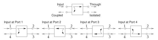
Figure 7-7: Directional coupler schematic drawn with each of the four possible input ports.
