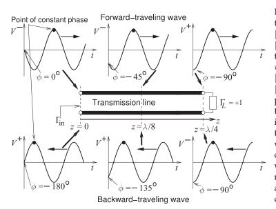
Figure 3-12: The forwardtraveling wave  $v^+(t,z)$  $|V^+|\cos(\omega t)$  $|V^+|\cos(\omega t + \phi(z))|$ the backward-traveling wave  $v^{-}(t,z) =$  $|V^+|\cos(\omega t)$  $|V^+|\cos[\omega t + \phi(z)].$ The phase,  $\phi$ , of the forwardtraveling wave becomes increasingly negative along the line as z increases, and when reflected the phase  $\phi$ of the backward-traveling wave becomes increasingly negative as the wave moves away from the load (i.e. as zdecreases).
