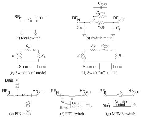
**Figure 11-12:** Microwave switches: (a) ideal switch connecting  $RF_{IN}$  and  $RF_{OUT}$  ports; (b) model of a microwave switch; (c) ideal circuit model with switch on and with source and load; (d) realistic low-frequency circuit model with switch on; (e) switch realized using a PIN diode; (f) switch realized using an FET; and (g) switch realized using a MEMS switch.
