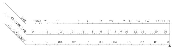
**Figure 8-4:** Nomograph relating the reflection coefficient (RFL. COEFFICIENT),  $\rho$ ; the return loss (RTN. LOSS) (in decibels); and the standing wave ratio (SWR).
