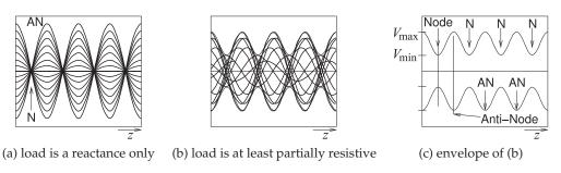
**Figure 3-14:** Standing waves as an overlay of waveforms at many times: (a) when the forward-and backward-traveling waves have the same amplitude; (b) when the waves have different amplitudes; and (c) the envelope of the standing wave. N is a node (a minimum) and AN is an antinode (a maximum). Nodes, N, are separated by  $\lambda/2$ . Antinodes, AN, are separated by  $\lambda/2$ .
