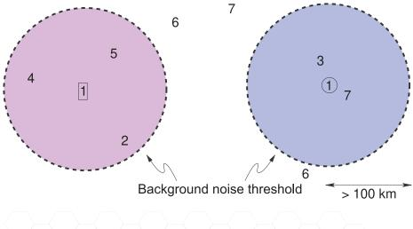
Figure 1-8: Interference in a conventional radio system. The two transmitters, 1, are at the centers of the coverage circles defined by the background noise threshold.
