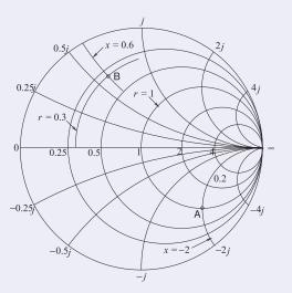
The impedance  $z_B = 0.3 + 0.6\jmath$  is plotted as Point B which is at the intersection of the circle r = 0.3 and the arc x = +0.6. Interpolation is required to identify the required circle and arc. The reader should do this with the full impedance Smith chart. As an exercise read off the reflection coefficient (the answer is  $-0.268 + \jmath 0.585 = 0.644 \angle 115^{\circ}$ ).
