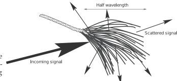
**Figure 2-14:** Pine needles scattering an incoming EM signal.
