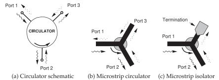
**Figure 11-16:** Ferrite components with a magnetized ferrite puck in the center in (b) and (c).
