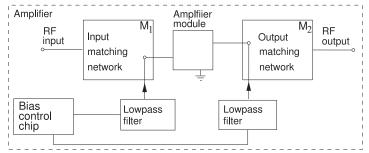
**Figure 11-5:** Block diagram of an RF amplifier including biasing networks.
