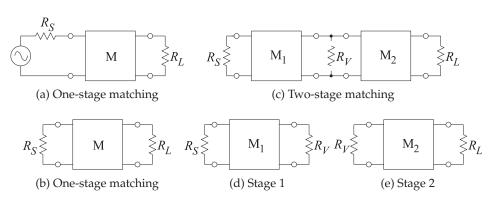
**Figure 10-18:** Matching in stages: (a) matching network M matching  $R_S$  to  $R_L$ ; (b) without an explicit source; (c) two-stage matching with a virtual resistor  $R_V$ ; (d) matching  $R_S$  to  $R_V$ ; and (e) matching  $R_V$  to  $R_L$ .
