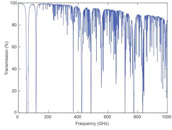
**Figure 1-1:** Atmospheric transmission at Mauna Kea, with a height of 4.2 km, on the Island of Hawaii where the atmospheric pressure is 60% of that at sea level and the air is dry with a precipitable water vapor level of 0.001 mm. After [1].
