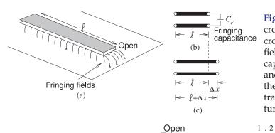
**Figure 9-11:** An open on a microstrip transmission line: (a) microstrip line showing fringing fields at the open; (b) fringing capacitance model of the open; and (c) an extended line model of the open with  $\Delta x$  being the extra transmission line length that captures the open.
