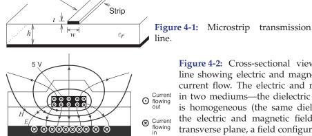
Figure 4-2: Cross-sectional view of a microstrip line showing electric and magnetic field lines and current flow. The electric and magnetic fields are in two mediums—the dielectric and air. If the line is homogeneous (the same dielectric everywhere) the electric and magnetic fields are only in the transverse plane, a field configuration known as the transverse electromagnetic mode (TEM).
