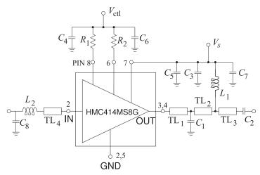
(b) Schematic of the evaluation board
