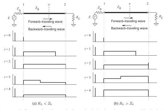
**Figure 3-9:** Reflection of a voltage pulse from a load: (a) when the resistance of the load,  $R_L$  is lower than the characteristic impedance of the line,  $Z_0$ ; and (b) when  $R_L$  is greater than  $Z_0$ .
