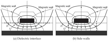
Figure 5-8: Approximate magnetic walls in microstrip where the *H* field is almost normal and the *E* field is almost parallel to the wall.
