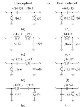
Figure 10-24: Four possible Pi matching networks: (a), (c), (e), and (g) conceptual circuits; and (b), (d), (f), and (h), respectively, their final reduced Pi networks.
