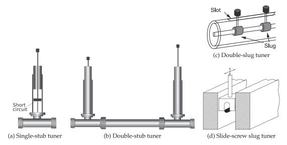
Figure 10-38: Laboratory tuners.
