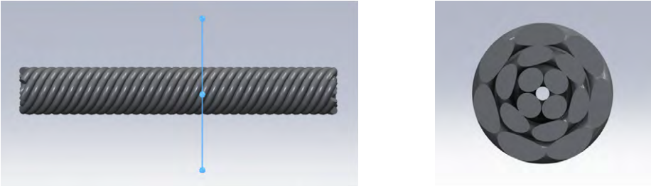
Figure 2.6: Cross section of the modelled yarn.
