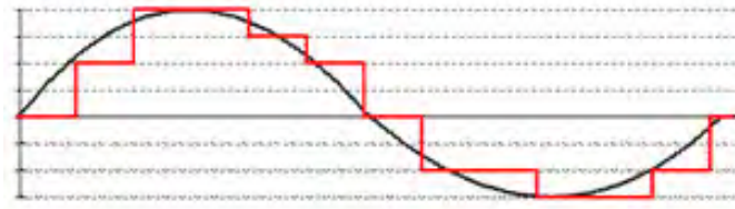
Figure 5.3: Continuous (black line) and discrete (red line) value sine-wave signal.
