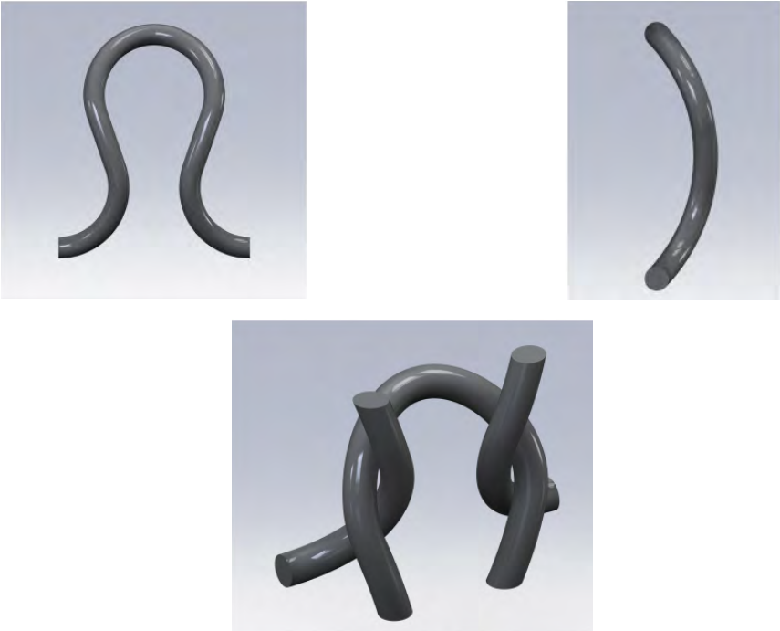
Figure 2.10: Modelling of the plain weft knitted loop and unit cell.
